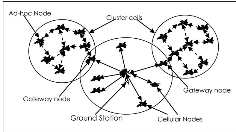
Figure 1: Mixed Network Architecture (source [1])
