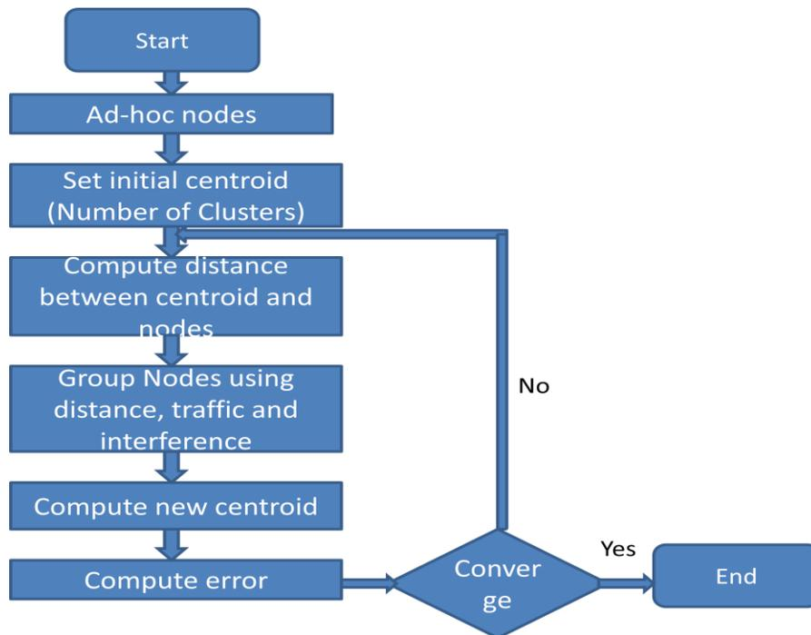
Figure 3: Clustering of Ad hoc Nodes, Stage two
