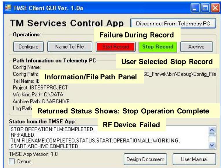
Figure 4: Standalone Control GUI
