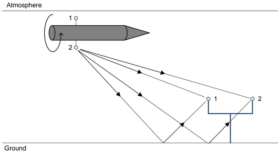
Figure 1 – Multiple Antennas Mounted on a Spinning Vehicle
