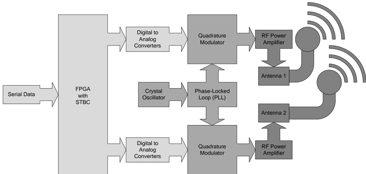
Figure 3 – MIMO Transmitter Block Diagram
