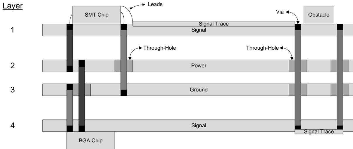
Figure 4 – PCB Cross Section
