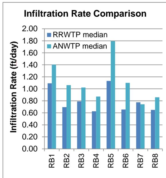
Figure 6. Comparison of median RRWTP Infiltration Rates (dark blue) compared to median ANWTP Infiltration Rates (teal) in RB-001 through RB-008
