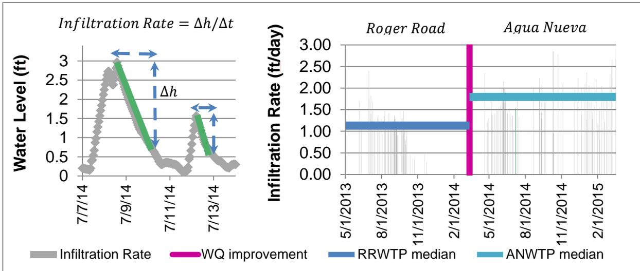
Figure 2. Sample infiltration calculations from SRF basin RB-005, including falling water levels collected by SCADA (left), and repeated many times to collect the median infiltration rate of the RRWTP (dark blue) vs ANWTP (teal) water
