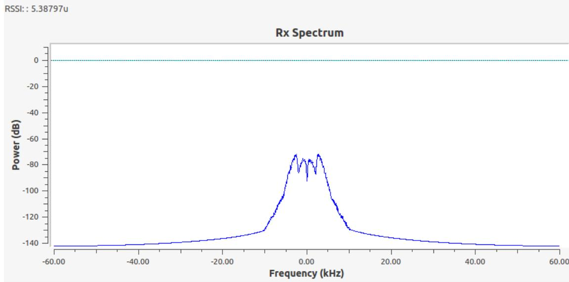
FIGURE 2: SAMPLE GFSK SIGNAL, AVERAGED, WITH CORRESPONDING AVERAGED RSSI VALUE.
