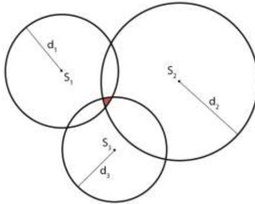
FIGURE 4: INTERSECTION POINTS FOR THREE BASE STATIONS, WITH THE ESTIMATED AREA OF ORIGIN FOR THE SOI COLORED IN RED.
