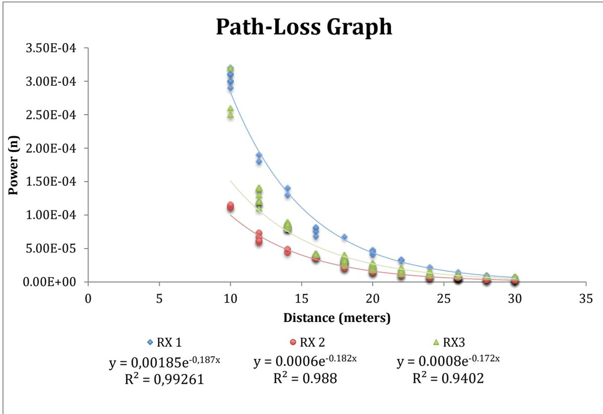
FIGURE 3: CURVE-FITTED PATH-LOSS EQUATIONS, BASED ON EXPONENTIAL REGRESSION, FOR THREE BASE STATIONS.
