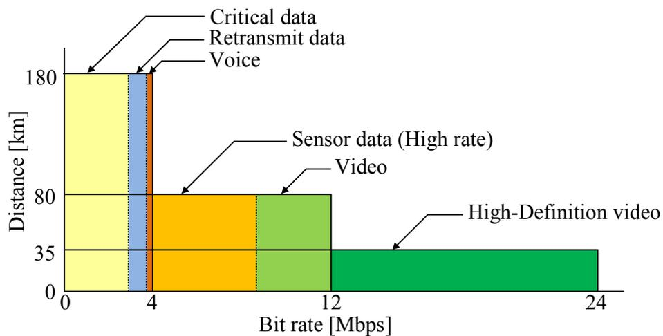
Figure 9 : Example of the transmission data priority
