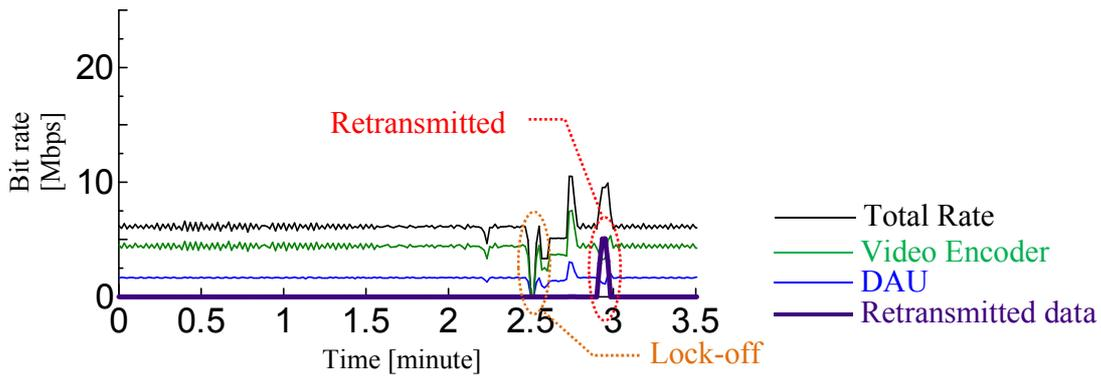
Figure 8 : The measurement data rate
