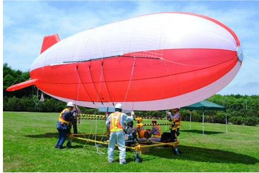
Figure 1 : The appearance of the tethered aerostat
