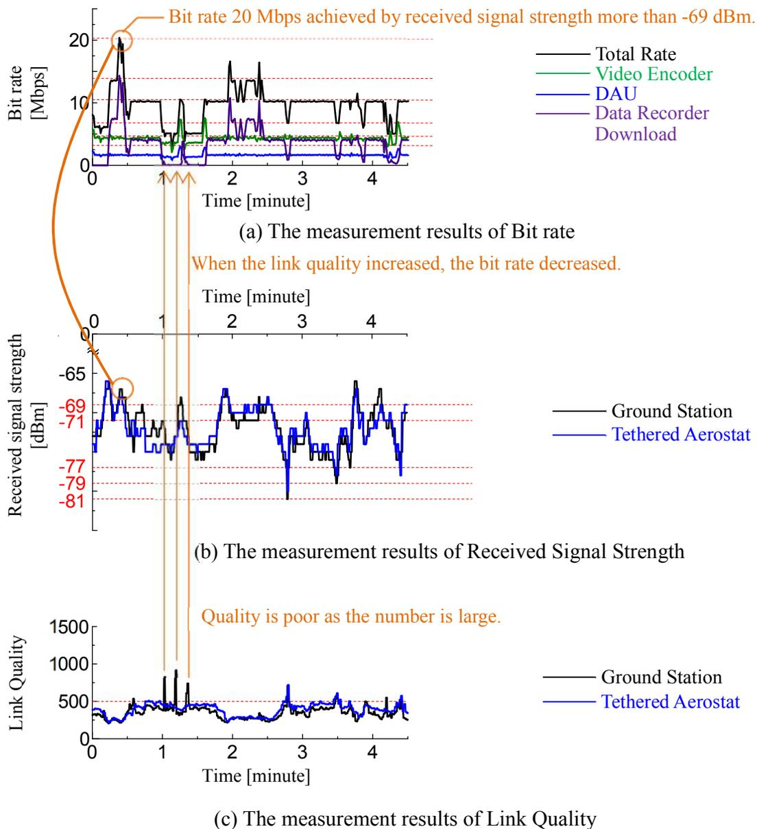
Figure 6 : The measurement results of Bit Rate, Received Signal Strength and Link Quality
