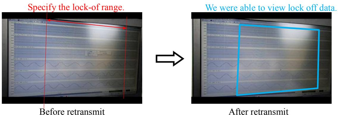
Figure 7 : The situation of lock-off data retransmit test
