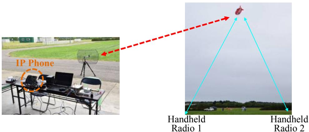
Figure 5 : Voice Communication Test Setup
