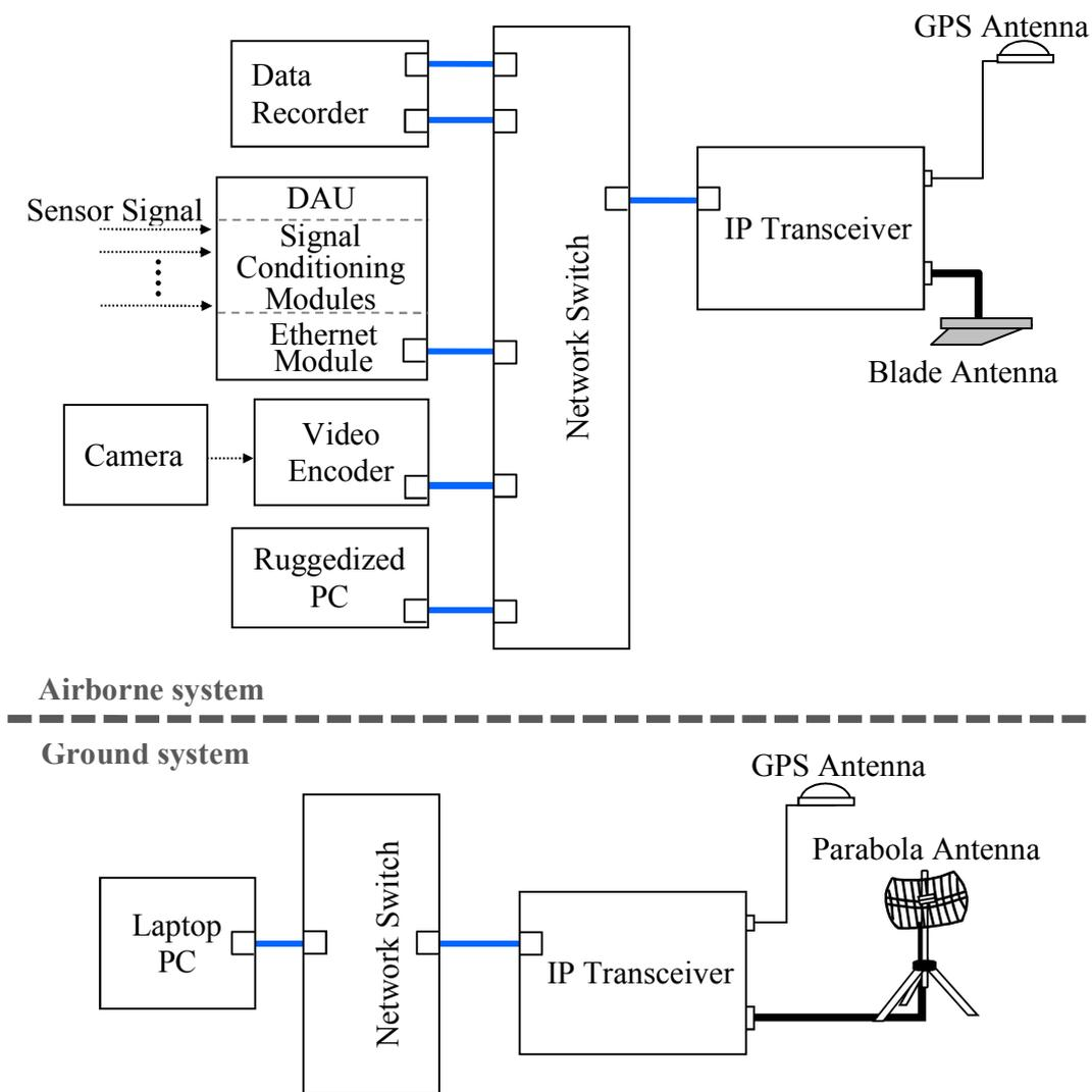
Figure 2 : System Configuration
