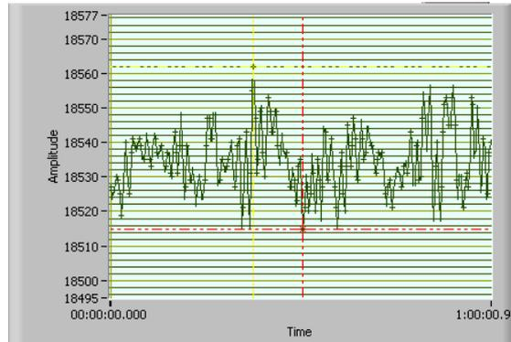
Figure 5: Zone B Dispersion for 10°C in instrument units given in number of converter of 16 bits.
