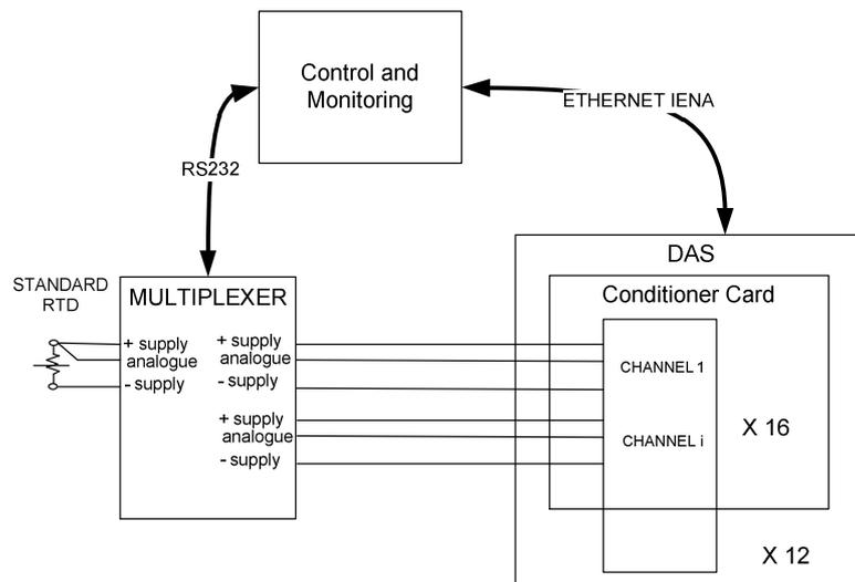
Figure 2: It shows the configuration of equipment to perform the calibration.
