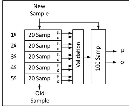
Figure 7: Shift register and validation criterion.
