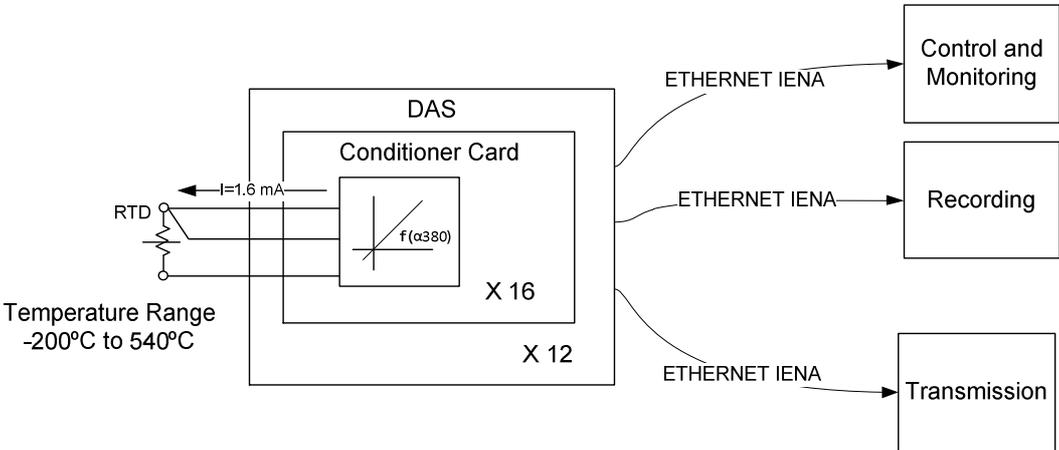
Figure 1: It depicts the instrumentation system; in particular the measurement chain for temperature.
