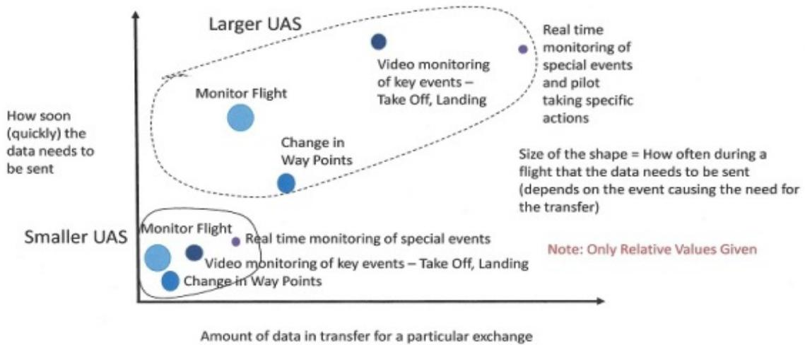
**Figure 7 Relative Information Transfers that could be needed during UA flights in the NAS**
