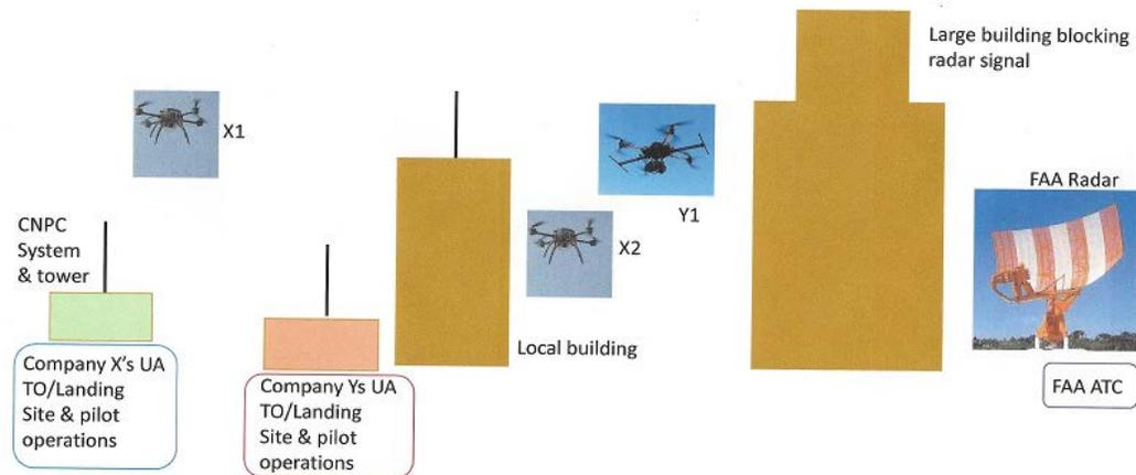
**Figure 4 sUAs conducting operations in an urban environment**
