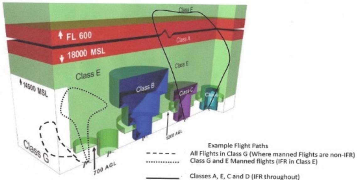
**Figure 2 U.S. Airspace Classes with 3 examples of UA flight paths superimposed**
