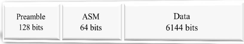
Figure 1: INET data packet structure
