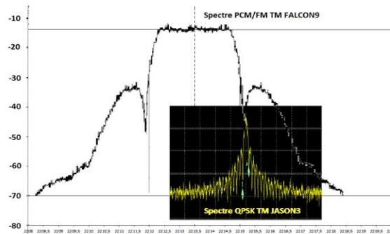
Figure 6. JASON3 and Falcon9 TM spectrums
