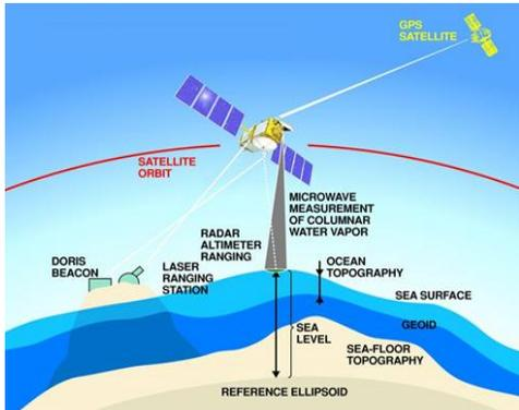
Figure 2. JASON3 Measurement System
