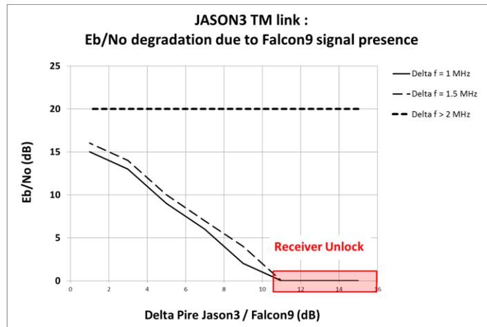
**Figure 7.  $E_b/N_0$  degradation on the JASON3 TM link**
