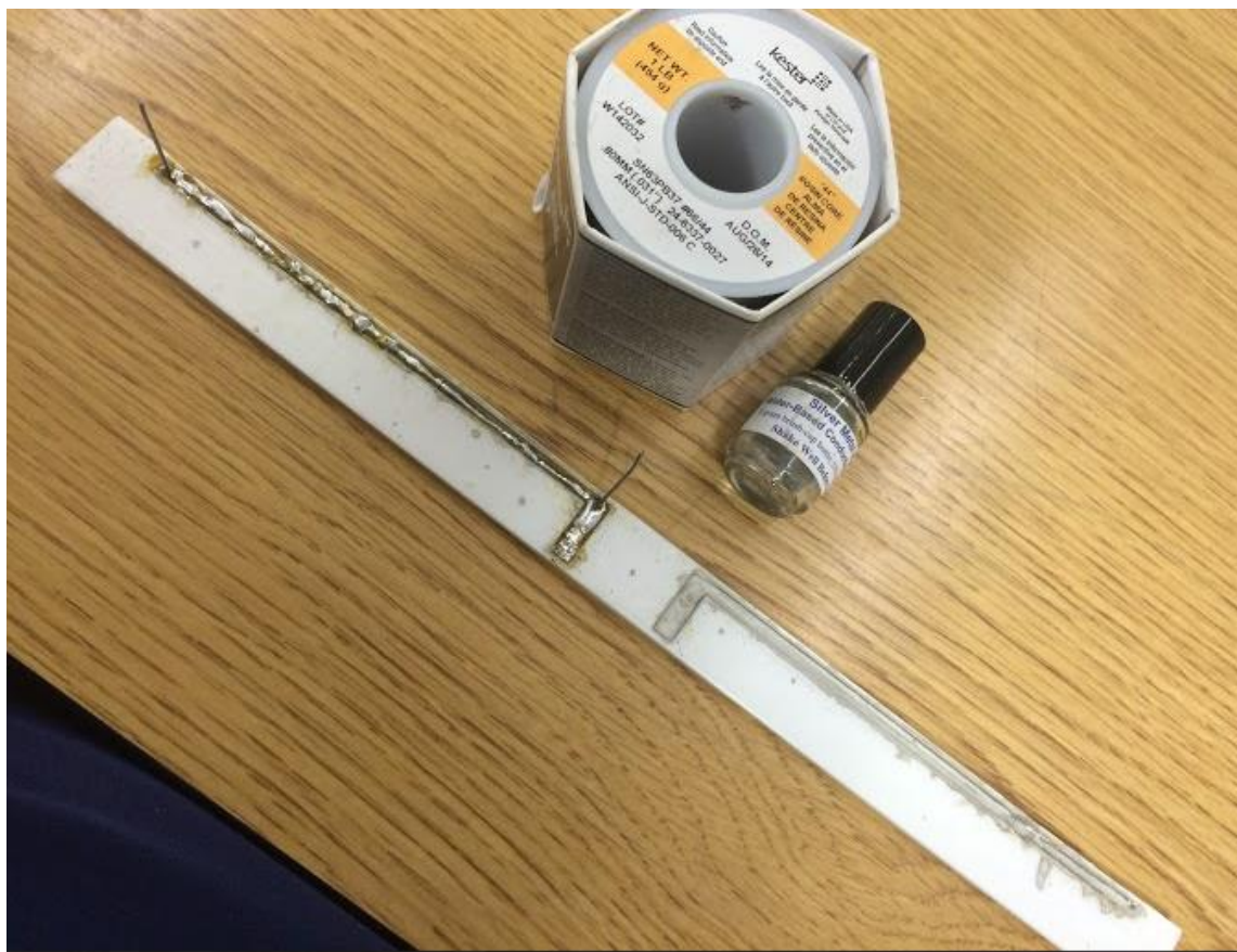
Figure 2: An antenna with one of the traces filled and the painted with conductive ink
