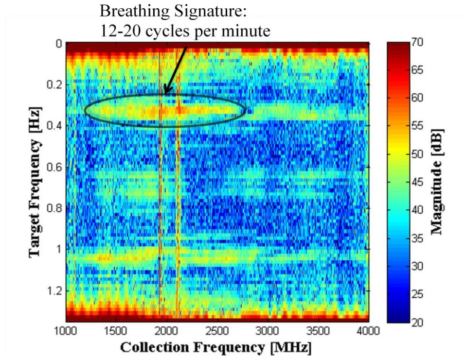
Figure 2: 2D Spectrum of Time Varying Range Profile  $P(f,k)$
