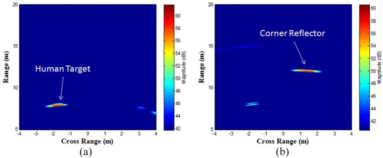
Figure 3: Back projection Imaging Results (a) Time-Varying Component and (b) Stationary Component
