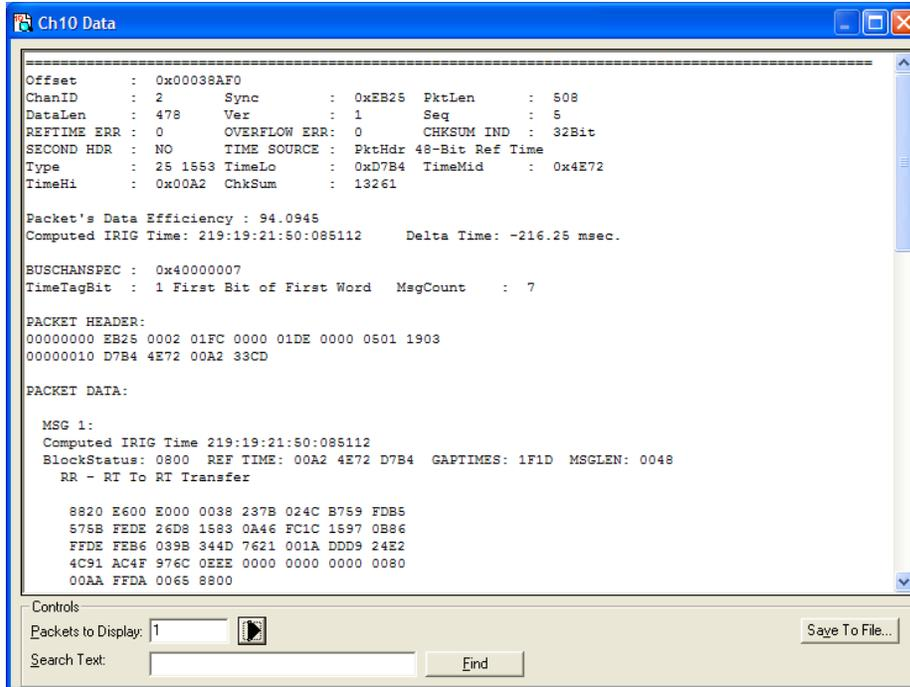
**Figure 1: Chapter 10 Packet Viewer – 1553 Bus Data Packet**
