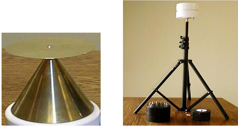
Figure (4): Discone omni-directional antenna for the microwave arrays.
