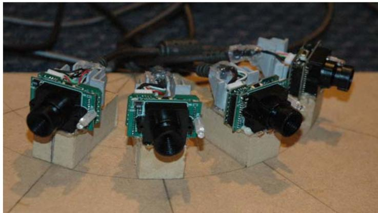
Figure (2-a): Multi-camera system for wide-angular coverage
