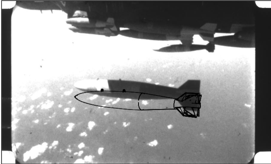
**Figure 4.** Digitized image of store with wire-frame model overlay
