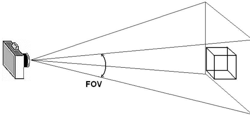
**Figure 2.** Lens calibration to calculate field-of-view
