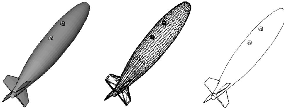
**Figure 3.** Solid CAD model (left), wire-mesh (center), silhouette (right)
