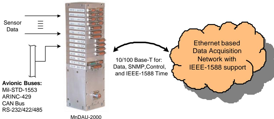
The heart of the network acquisition unit is its built-in Power PC processor and its peripherals. The design approach was to devise an architecture that allows for maximum flexibility and capabilities that would have been unimaginable just a few years ago. The architecture shown in Figure 2 includes four core functions to enable data acquisition and automatic format generation:
