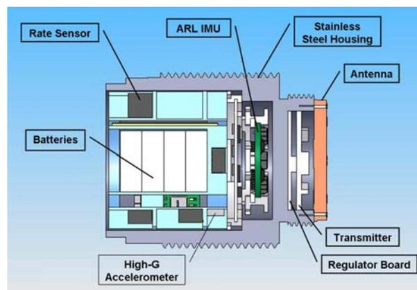
Figure 6 – Apollo CEV Telemetry Module Cutaway View
