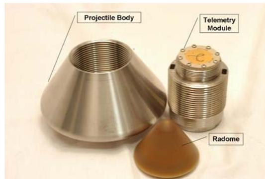
Figure 4 - Instrumented CEV Round Components
