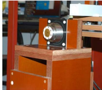
Figure 9– Magnetometer Calibration Setup
