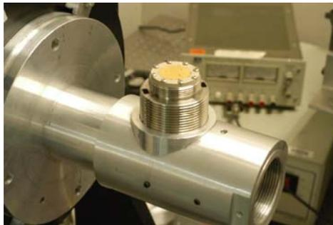
Figure 7 – Accelerometer Calibration Setup
