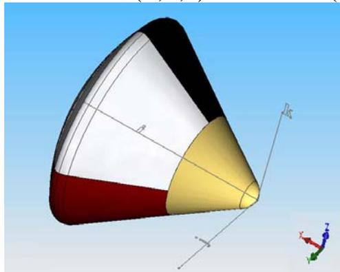
Figure 14 – Coordinate System for Apollo CEV
