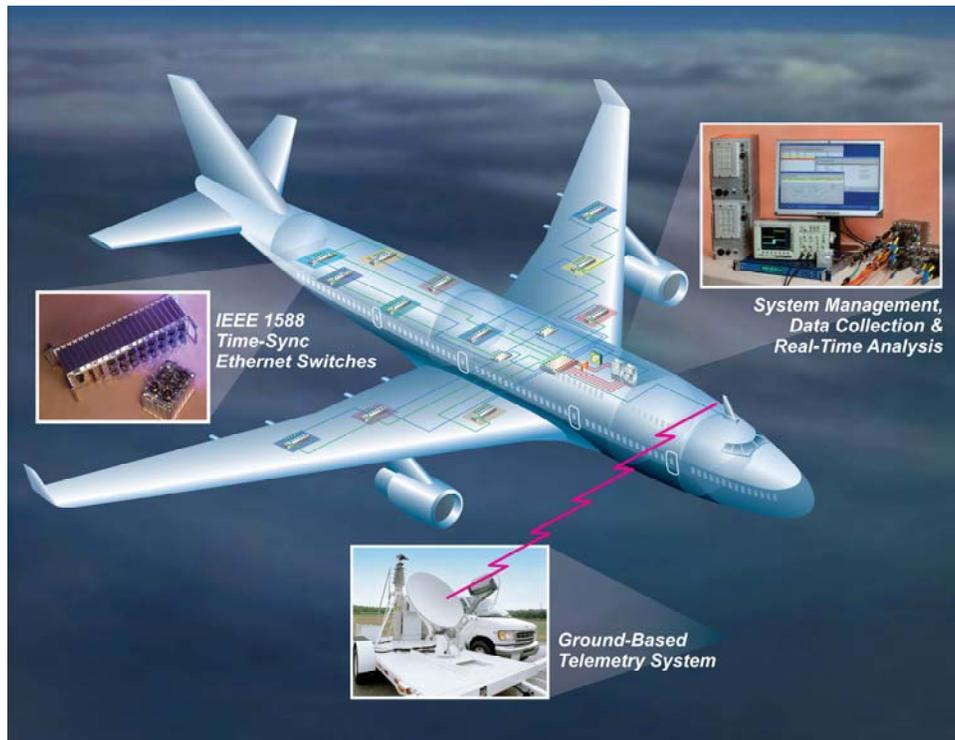
**Figure 5. Network-Enhanced Data Acquisition and Telemetry System**
