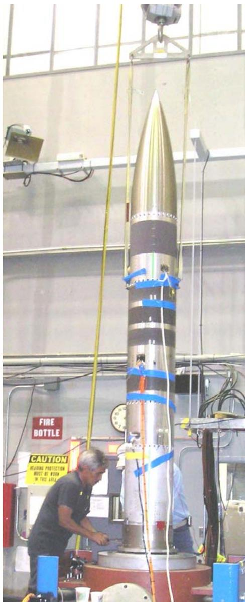
**Figure 4: Vertical Vibration Test**
