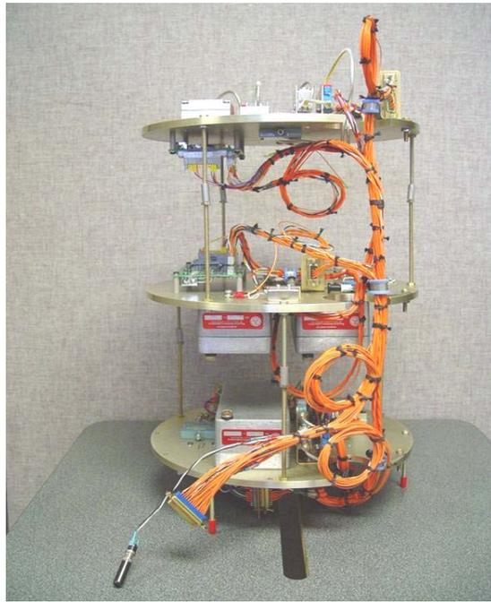
**Figure 2:** 2 PRBS Generators, 3 S-band Tx's, S-to-X-band up converter and PA, and Batteries
