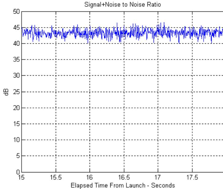
**Figure 12:** TGRS S-band (Signal + Noise)/Noise Measured at the 30-foot Antenna
