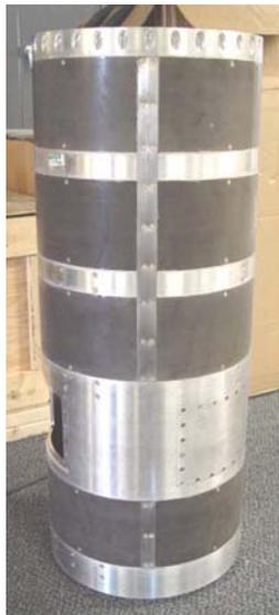
**Figure 1b:** Payload Antennas for X-band Tracking and S-band Modulation Comparison
