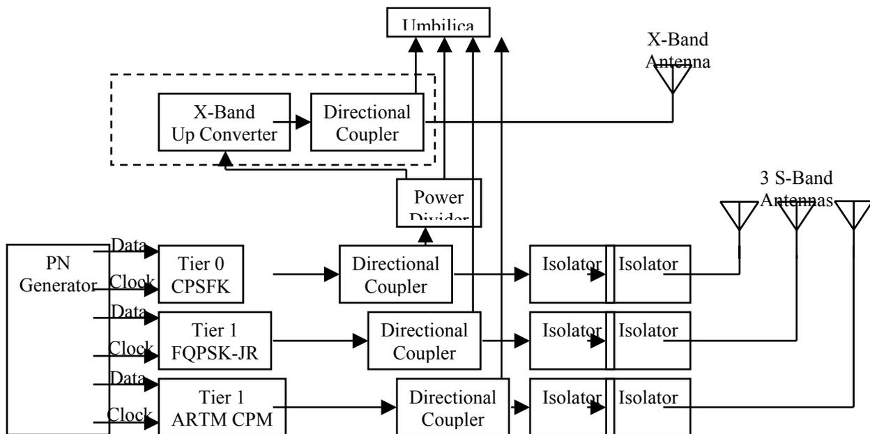
**Figure 1a:** Payload Antennas for X-band Tracking and S-band Modulation Comparison
