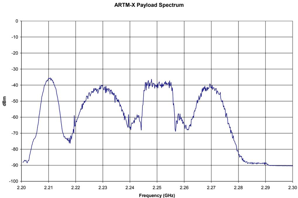
**Figure 5:** Four S-band Transmitters with Translated GPS, CPM, FM and SOQPSK
