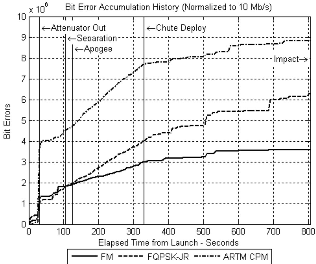
**Figure 13: S-band Bit Error Accumulation History Measured at the NASA 30-foot Antenna**
