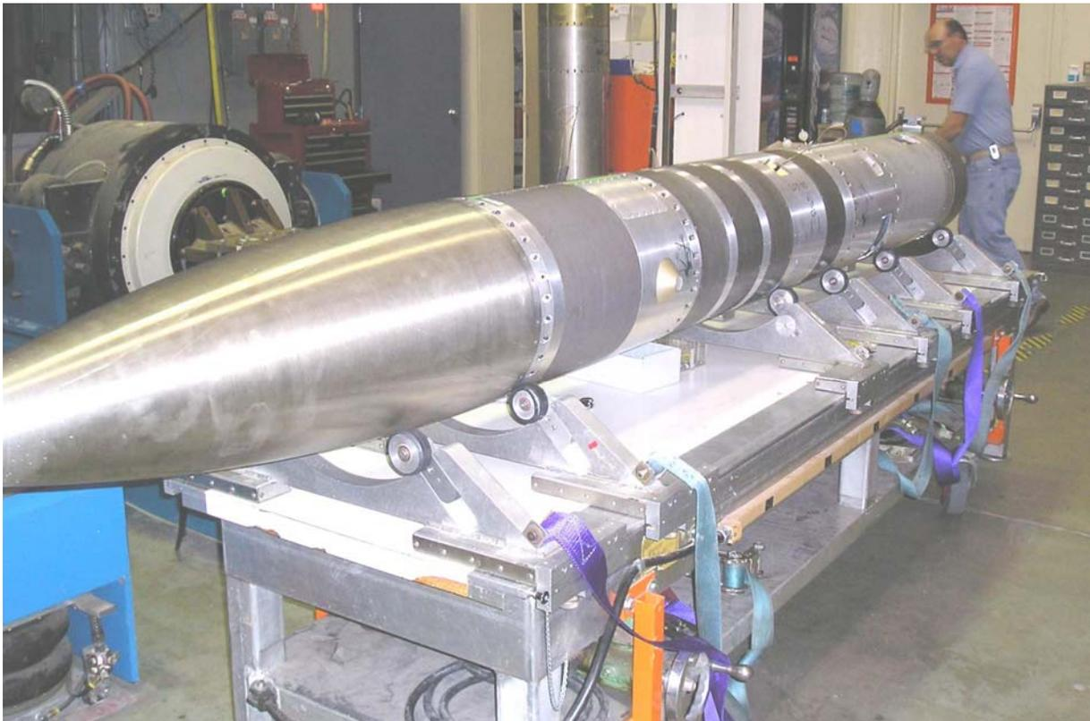
**Figure 3:** Nosecone, Primary Translated GPS Payload, X-band Antenna and 3 S-band Antennae Piggyback Payload for Modulation Comparison-Parachute Recovery System
