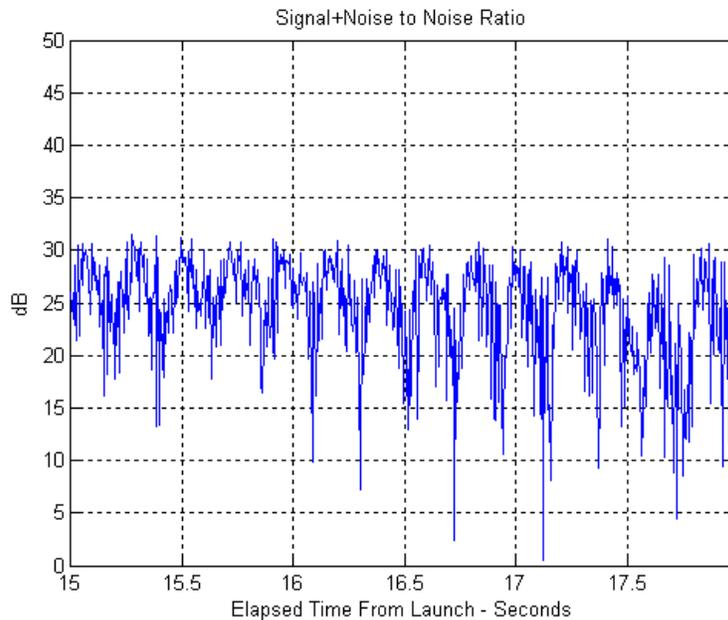
**Figure 11:** X-band Spin Rate Fades in (Signal + Noise)/Noise Measured at the 8-foot Antenna
