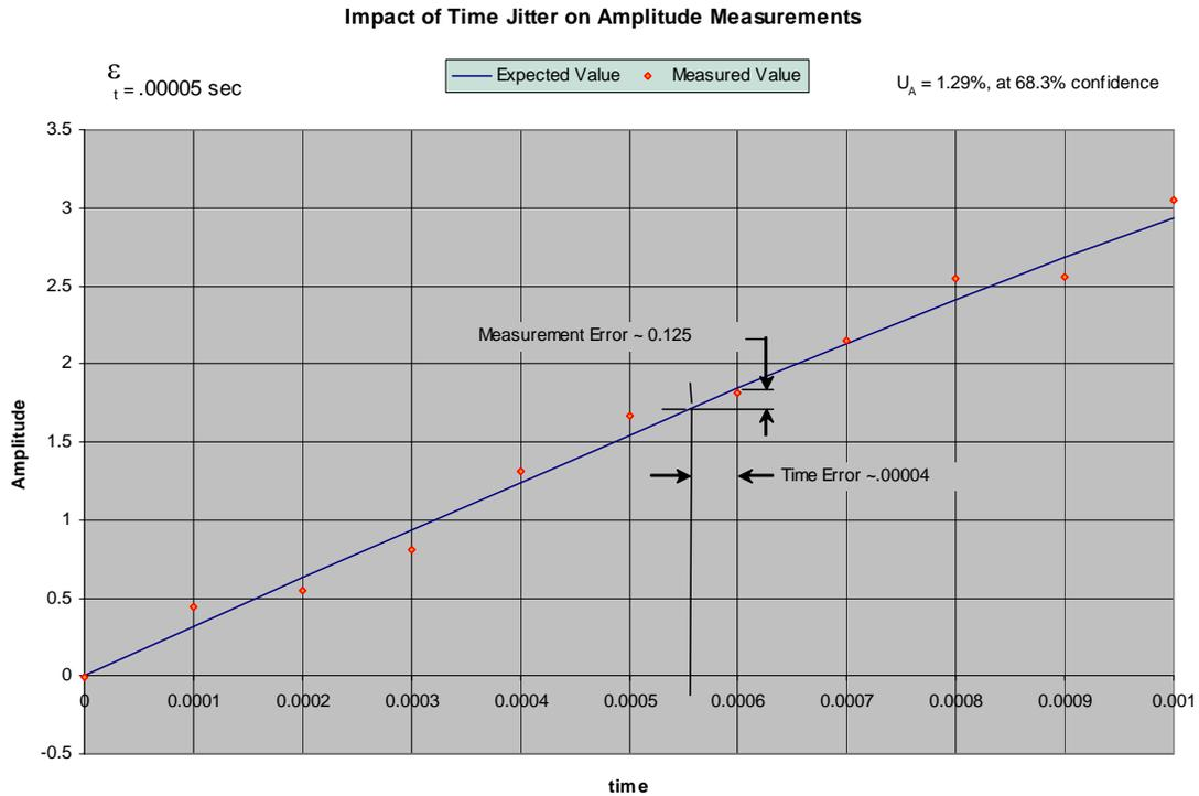
**Figure 2 Effect of Time Jitter on Amplitude Measurements**
