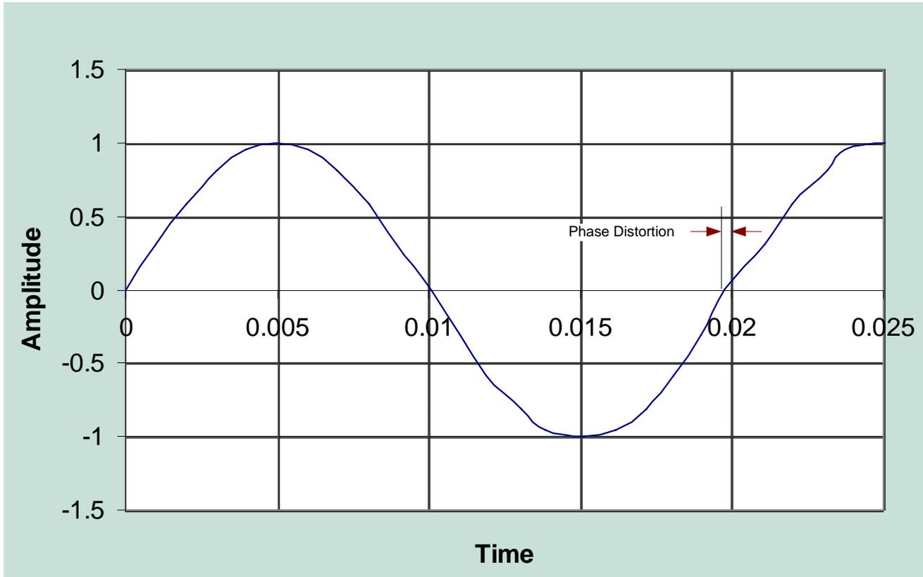
**Figure 1 Sample Time Error Caused Phase Distortion**
