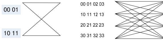
Figure 5: 2 state binary STTC encoder vs. 4 state 4-ary STTC encoder for 2 transmit diversity
