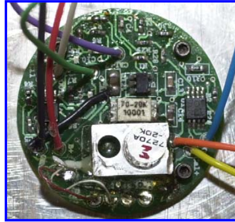
Figure 4: Accelerometer Test Board
