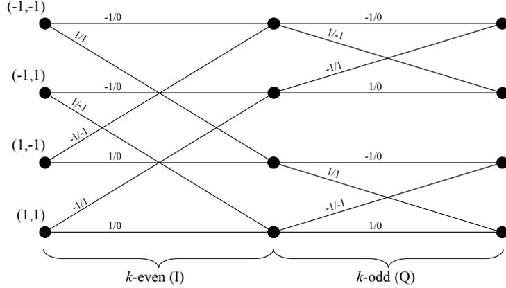
Figure 1: Four state trellis diagram for SOQPSK.
