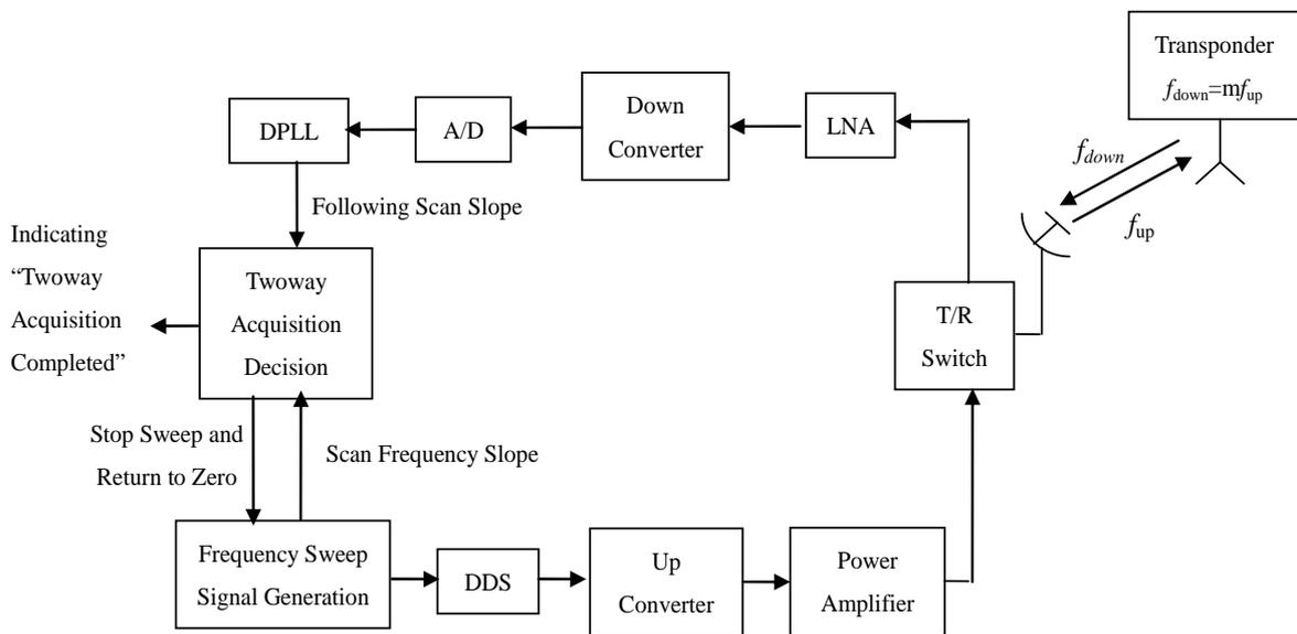
**Figure 1 Frequency Scan/Following Scan Twoway Acquisition Block Diagram**
