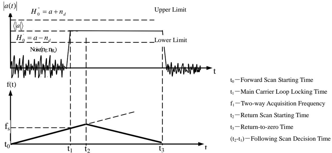
**Figure 4 Two Thresholds Decision Waveform Diagram**
