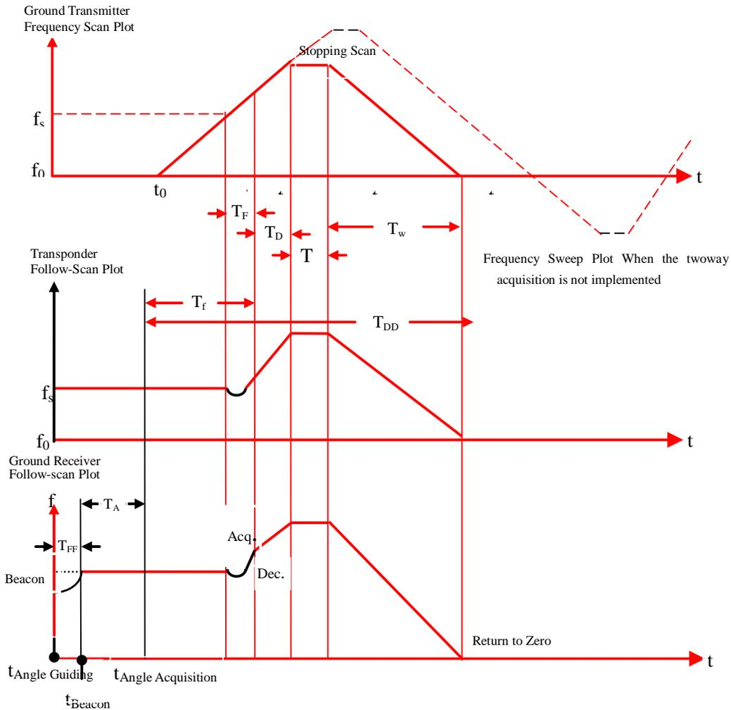
**Figure 5 Twoway Acquisition Process Chart**
