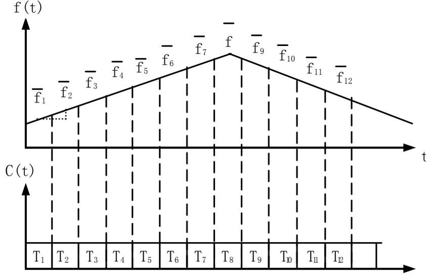
**Figure 2 Allan Variance Calculations for Linear Frequency Scan**
