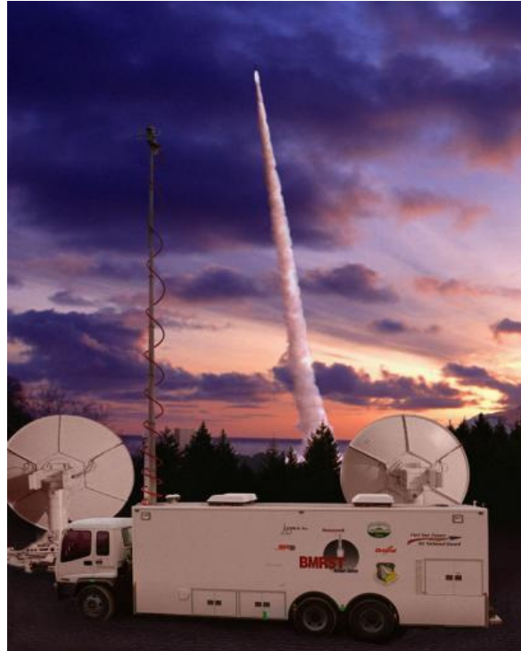
Figure 1 Two opposite circular polarized antennas tracking a launch
