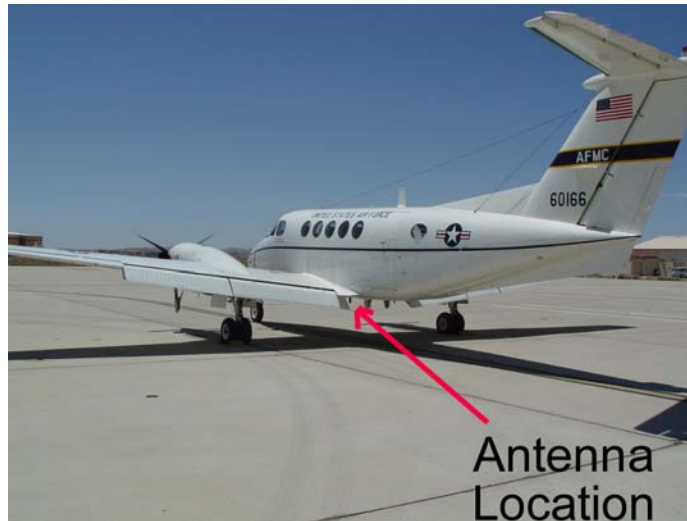
Figure 2 – Aircraft Antenna Installation Location
