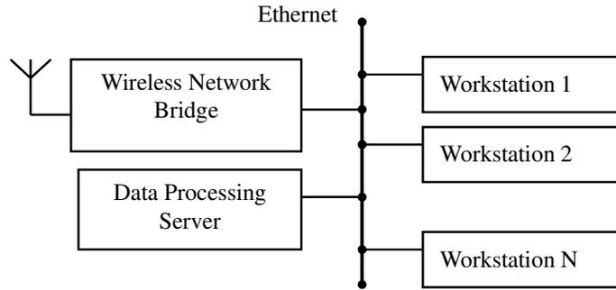
Fig. 1b Block Diagram of the Ground Part of the Wireless Network-based rfNET for Flight Test
