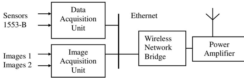
Fig. 1a Block Diagram of the Airborne Part of the Wireless Network-based rfNET for Flight Test
