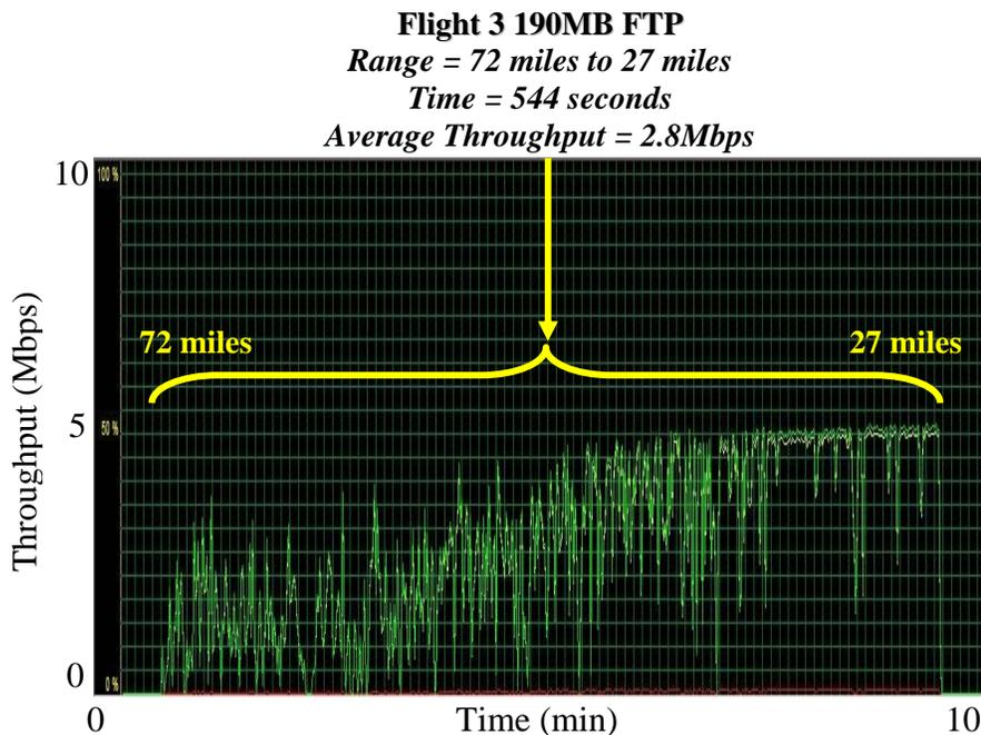
Figure 2. Flight 3 FTP transfer with decreasing range.
