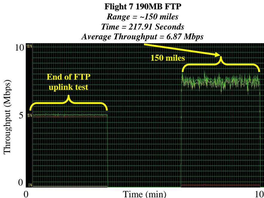
Figure 3. Flight 7 FTP transfer at 150-mile range.
