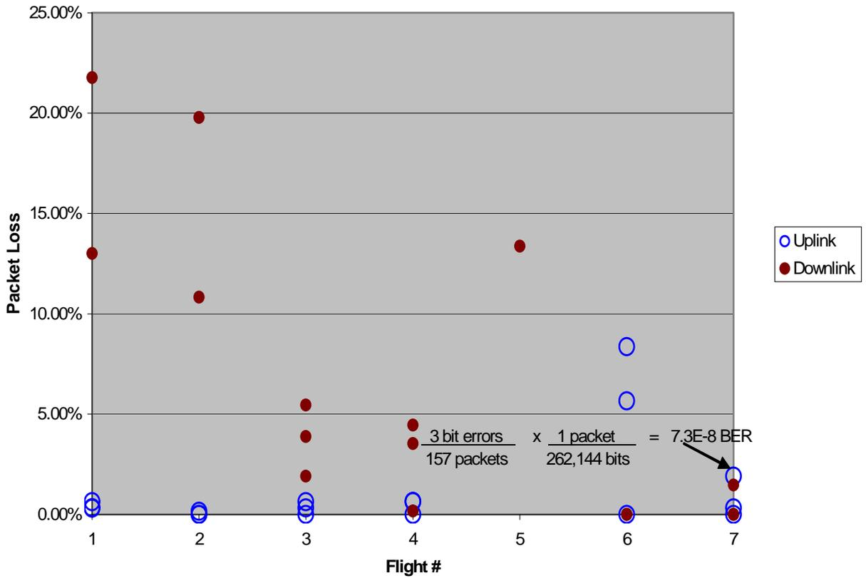
Figure 7. Iperf-measured UDP packet loss vs. flight number.
