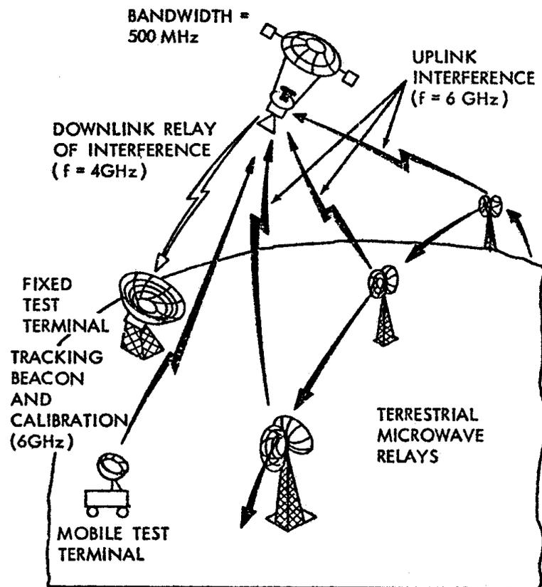
**FIGURE 1. 6 GHz RFI Experiment**
