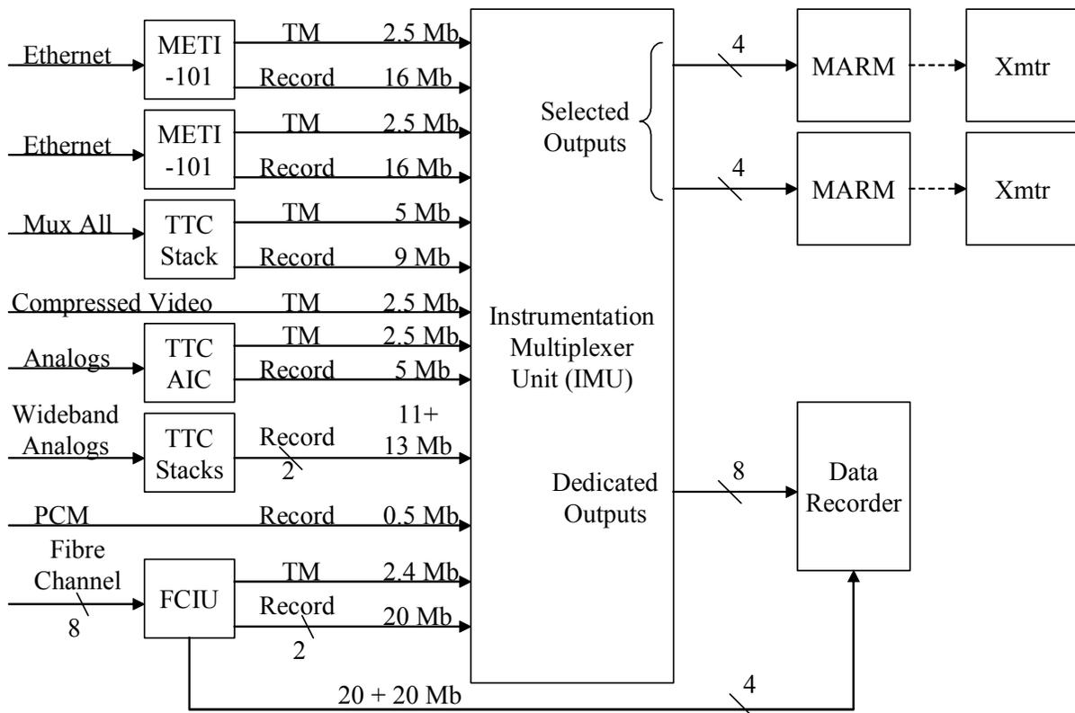
**Figure 3. Recorded and Telemetered PCM Streams**
