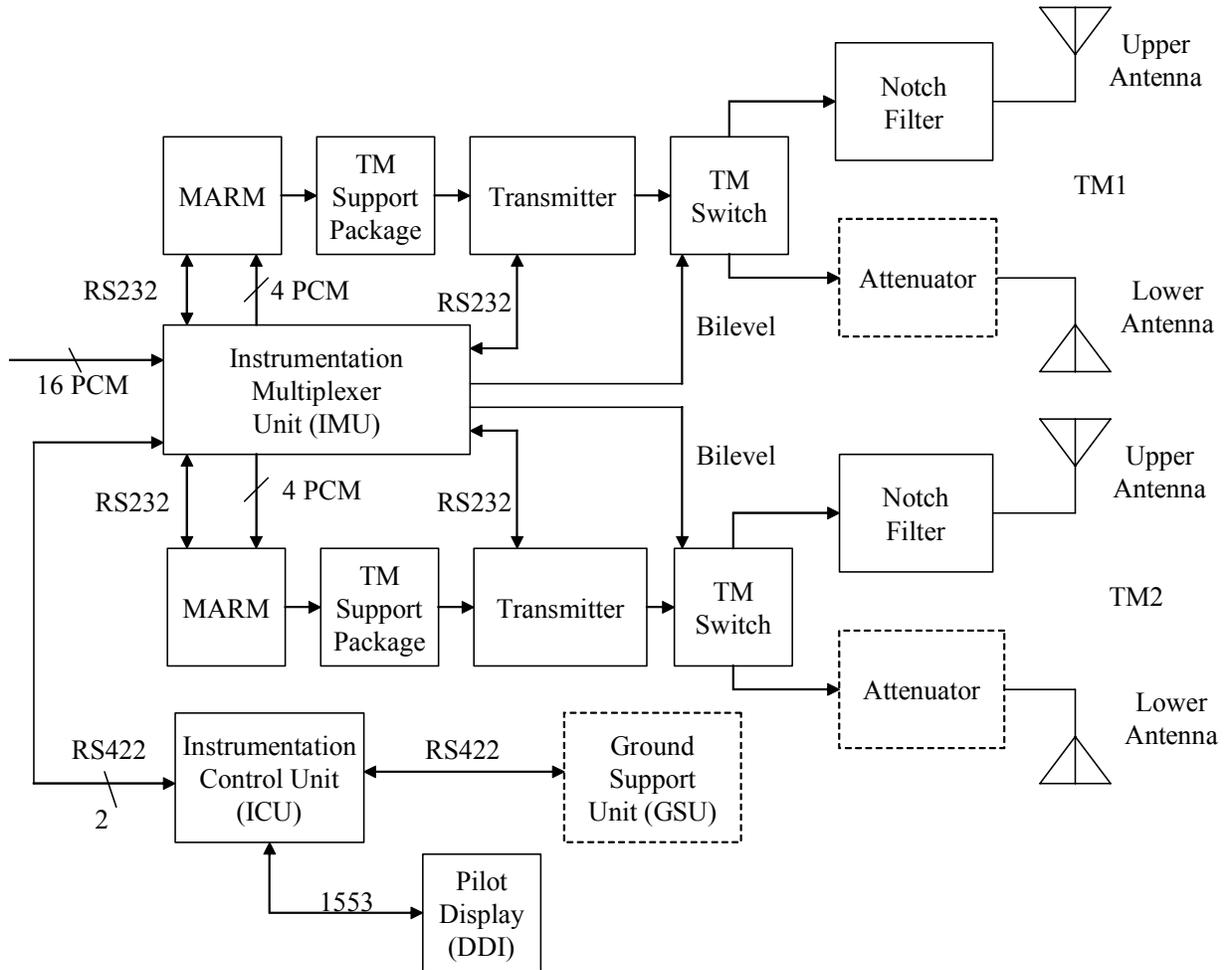
**Figure 1. Telemetry System Block Diagram**
