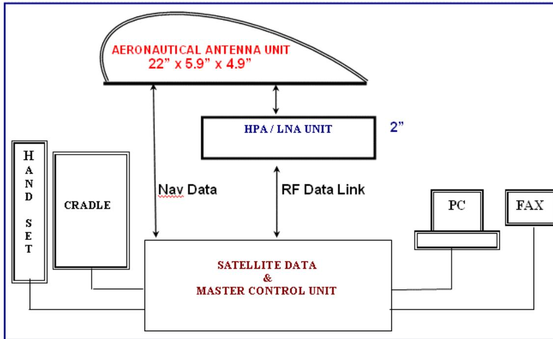
Fig.5: Configuration of the air mobile communication link
