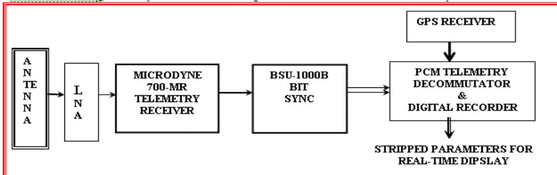
**Fig.3 : Configuration of Telemetry Chain**
