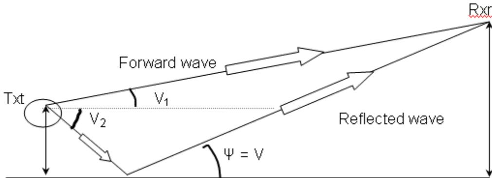
Fig.10: Geometrical relations during multipath
