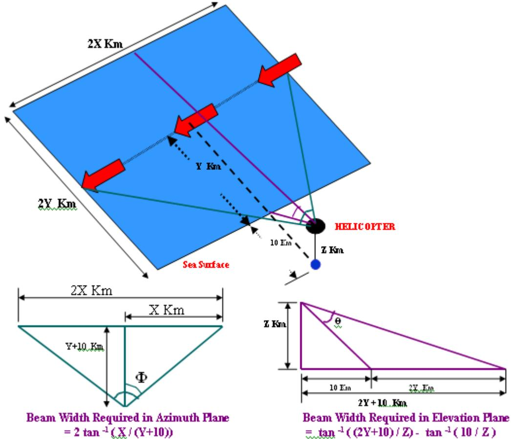
Fig.1 : Terminal phase coverage requirements
