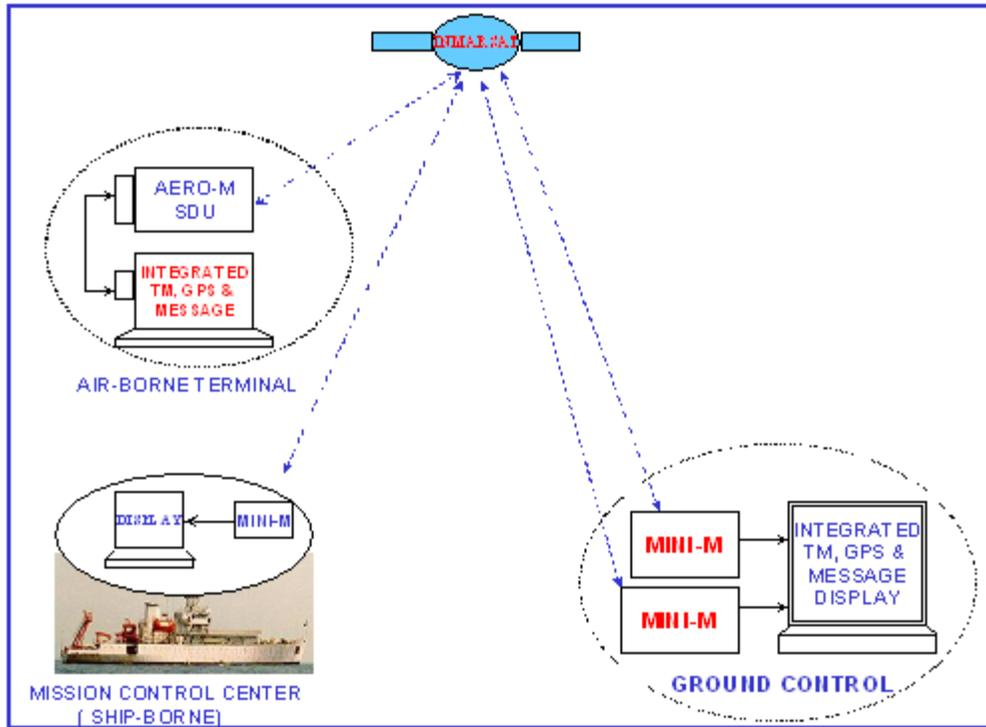
Fig.6: Realization scheme of air mobile communication link
