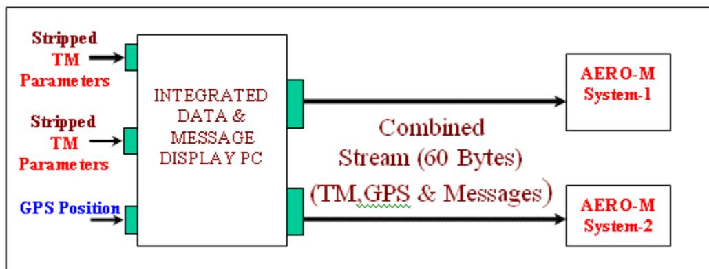
Fig.7 : Integrated display configuration on-board helicopter
