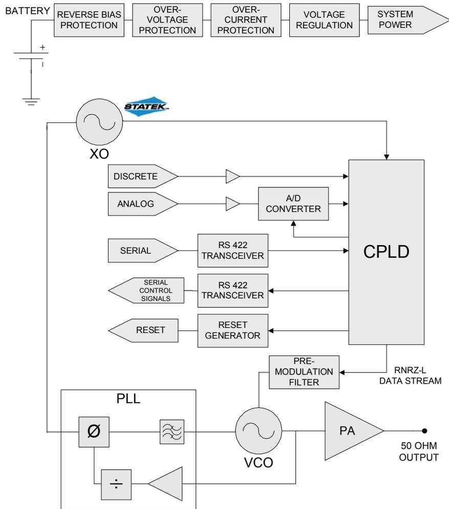
**Figure 1 – TTM System Block Diagram**
