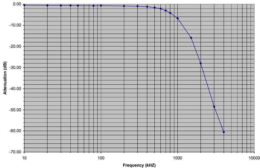
**Figure 2 – Frequency Response of Pre-Modulation Filter**
