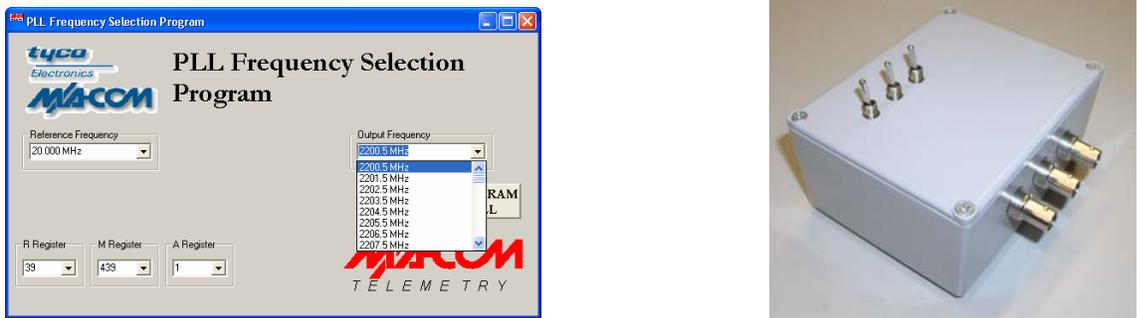
**Figure 4 – M/A-COM GUI and Programming Box**
