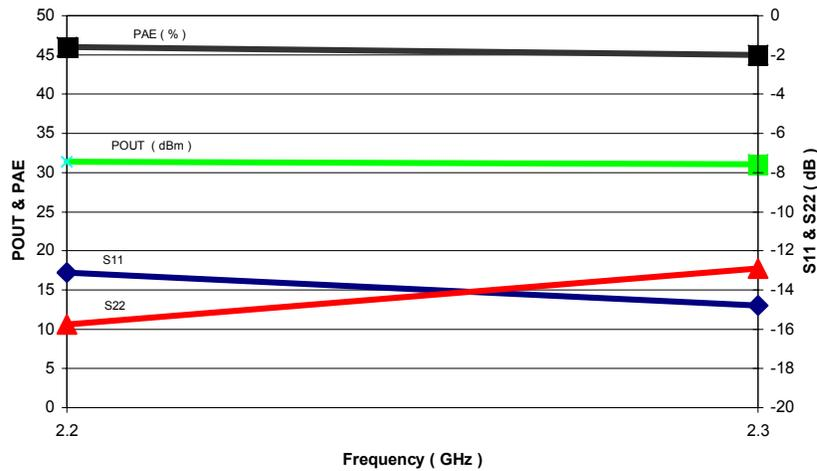
**Figure 3 – Measured performance of the 1 W MMIC HPA @  $V_{DS} = 5.0V$**
