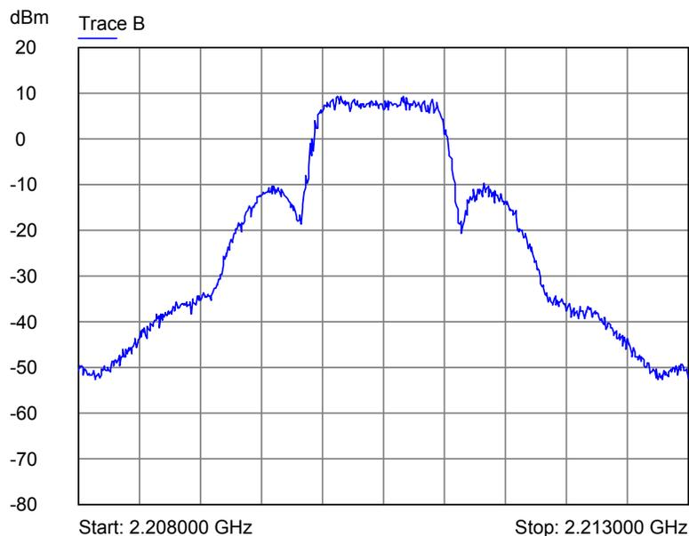
**Figure 5 – TTM Modulated RF Output Spectrum**
