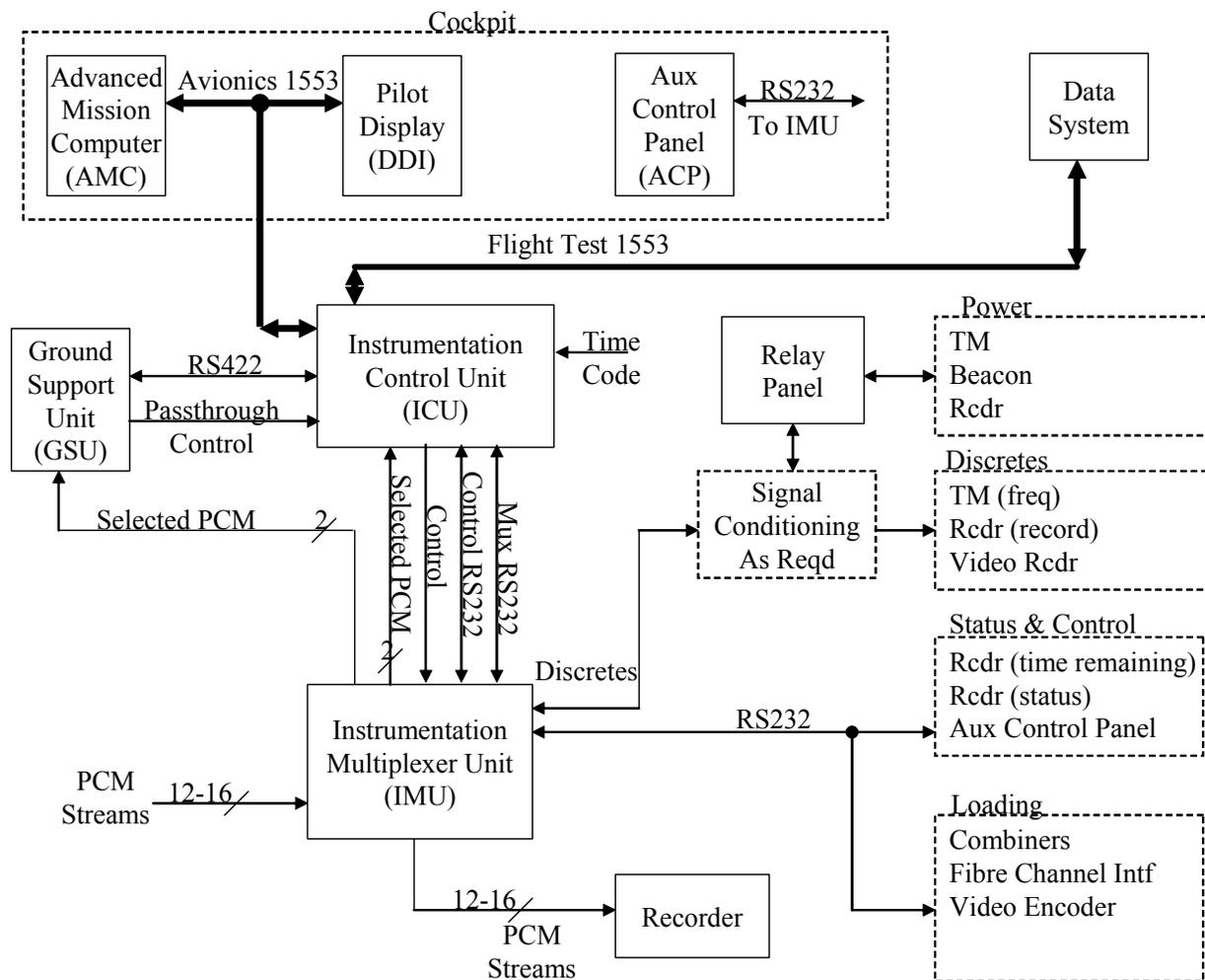
**Figure 1. Instrumentation Control System EA-18G Aircraft Configuration**
