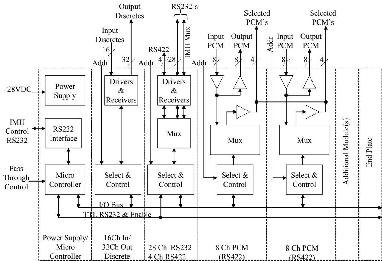
**Figure 4. IMU Block Diagram**
