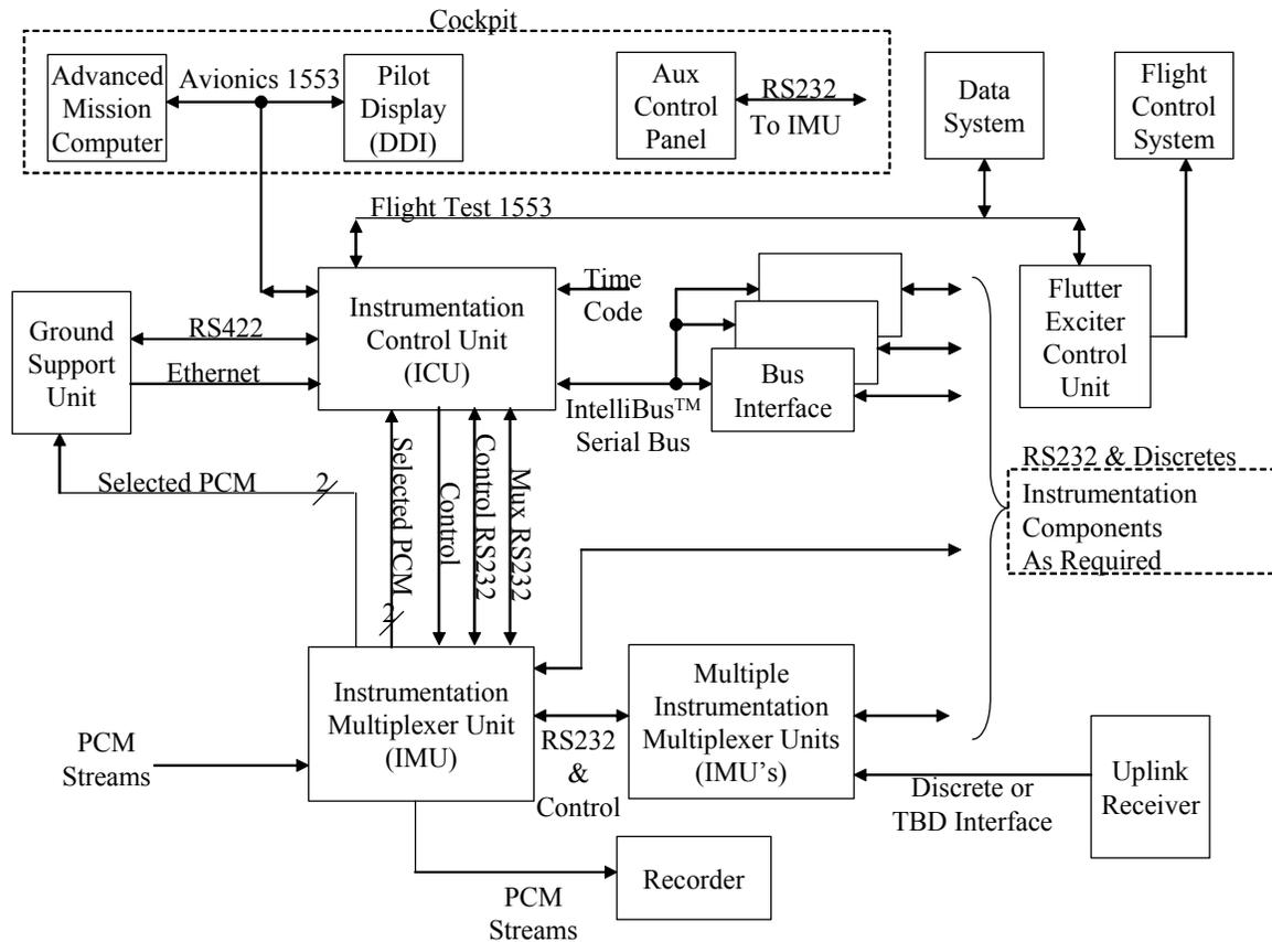
**Figure 5. Advanced System Capabilities**
