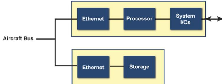
Figure 4 Storage in a distributed system
