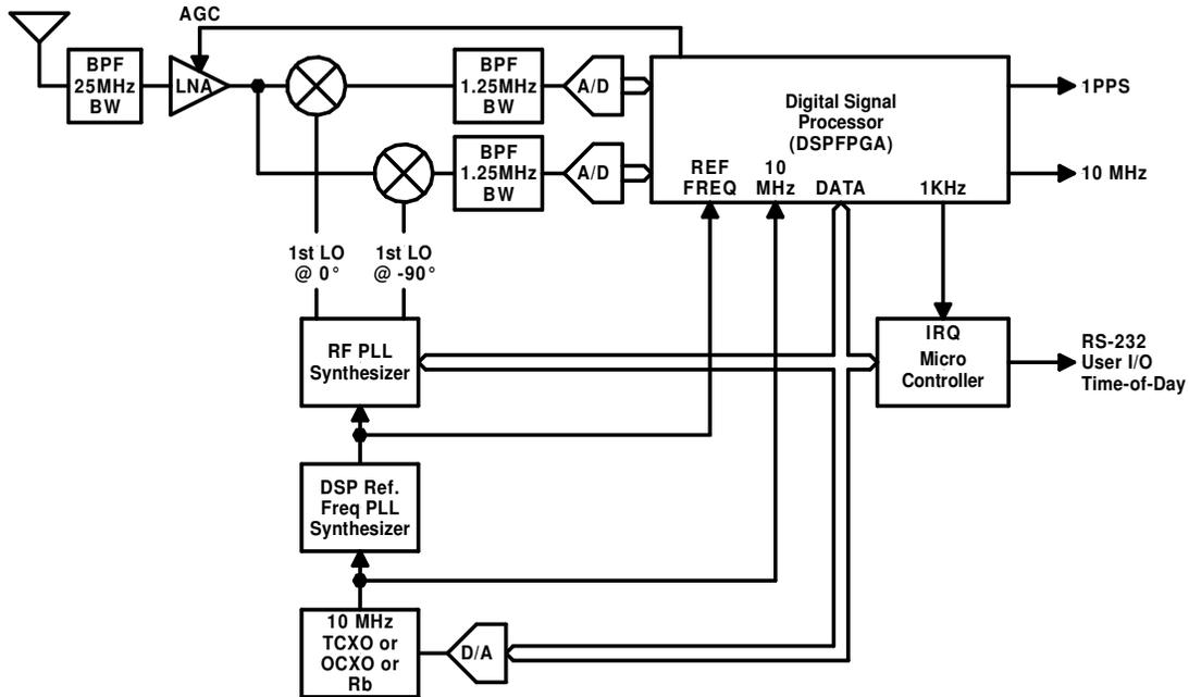
**Figure 3 – CDMA Time and Frequency Receiver**
