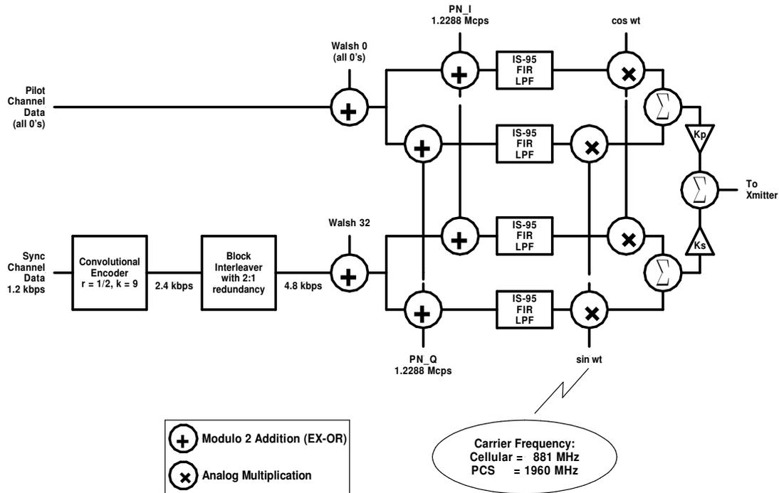
**Figure 2 – Pilot and Sync Channel Signal Structure**
