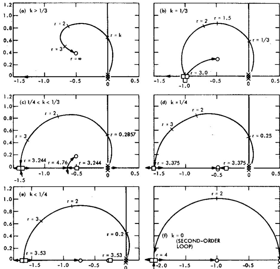
Fig. 4 - Root loci of the third-order as a function of  $r = AK\tau_2^2/\tau_1$  for various values of the parameter  $K = \tau_2/\tau_3$
