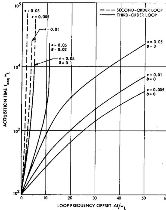
Measured acquisition time as a function of loop frequency offset (normalized axis)
