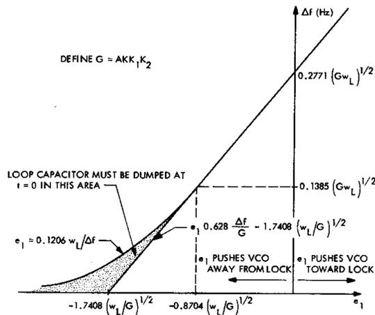
Fig. 3 - Maximum initial frequency detuning  $\Delta f(\text{Hz})$  for which a third-order loop pulls to zero-beat, as a function of the phase-detector/operational amplifier bias imperfection  $e_1$  (normalized by the peak S-curve value)
