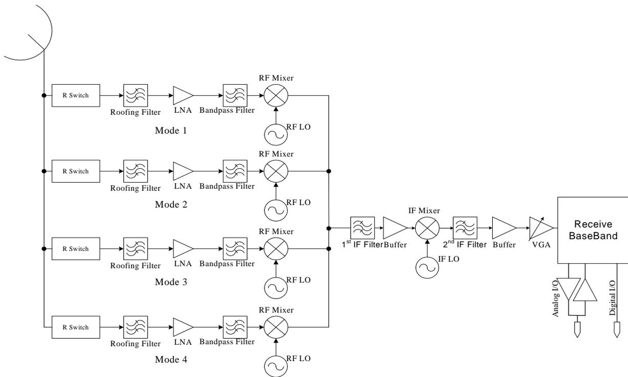
Fig. 1: Multiple RF Front-end Receiver
