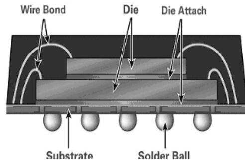
Fig. 7: Multichip Stack
