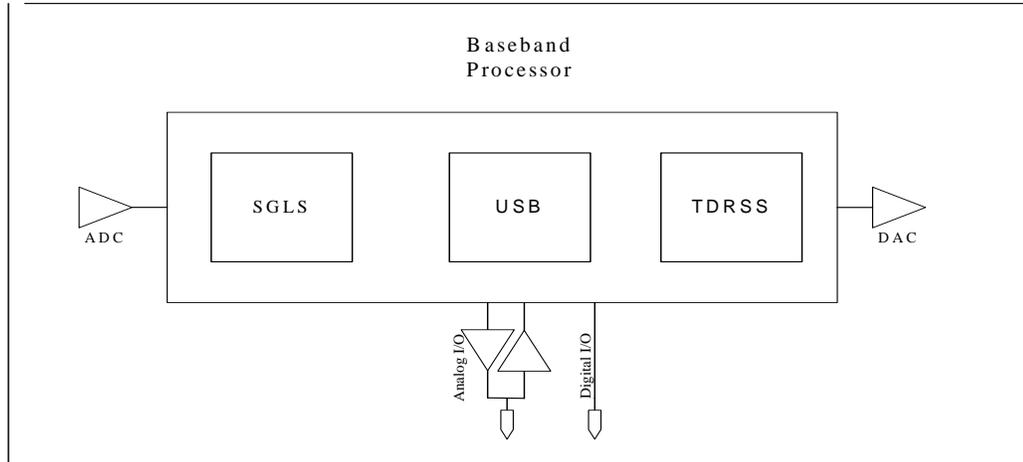
Fig. 4: Parallel Resident Waveform Baseband Architecture
