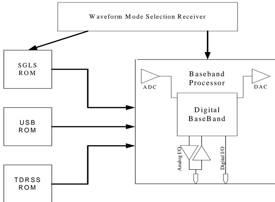
Fig. 3: PROM-Based FPGA Receiver Design
