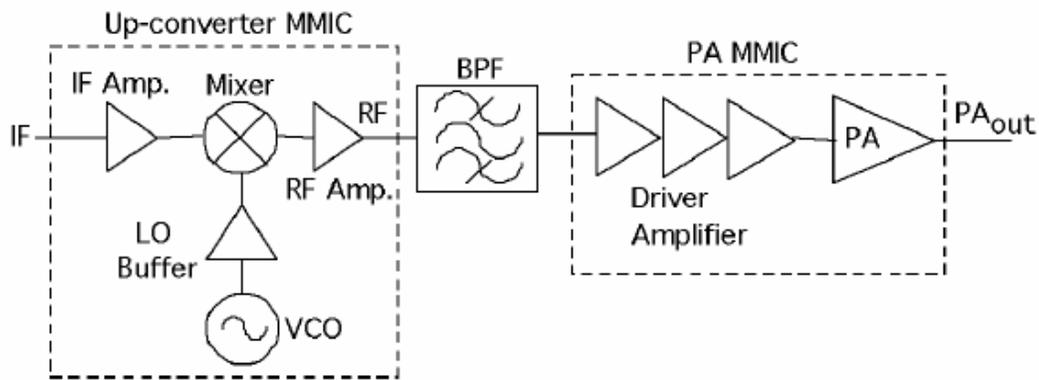
Fig. 2: Up Conversion at Ku and Ka Bands[7]
