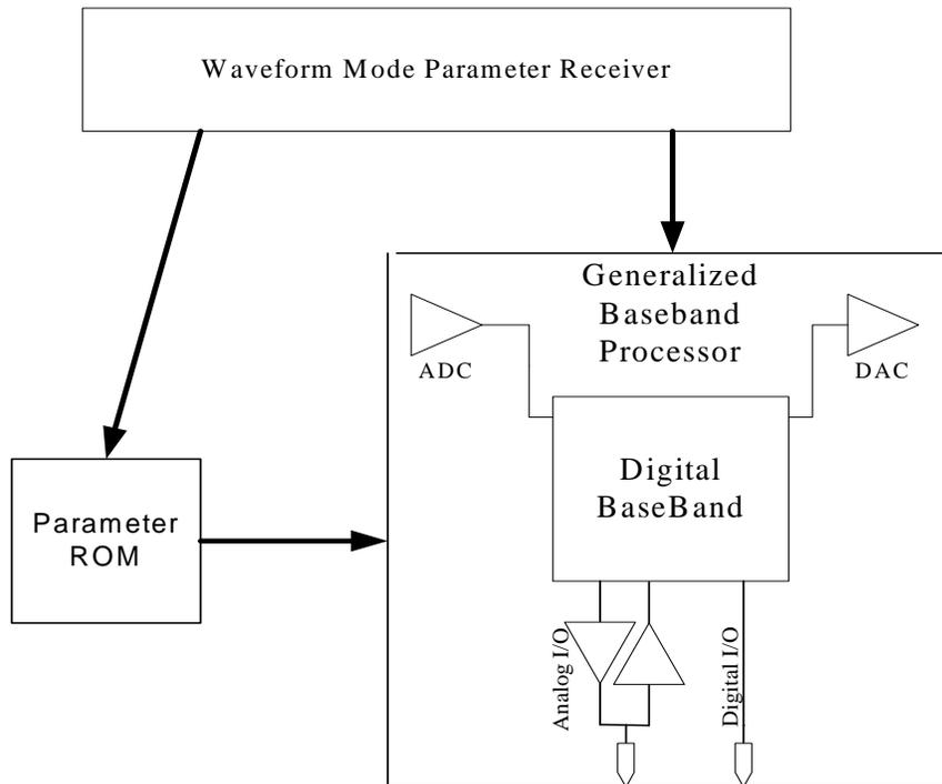
Fig. 5: Parameter Based Baseband
