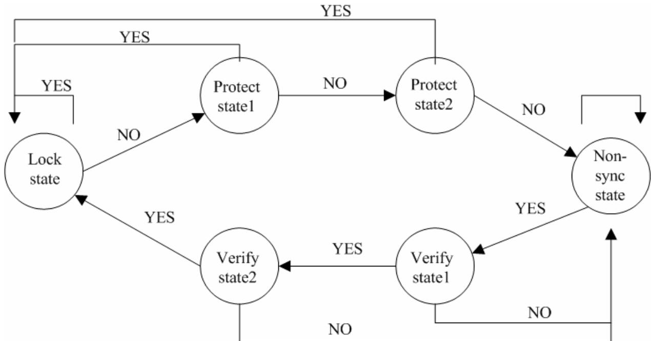
Figure 6 the State Convert Diagram
