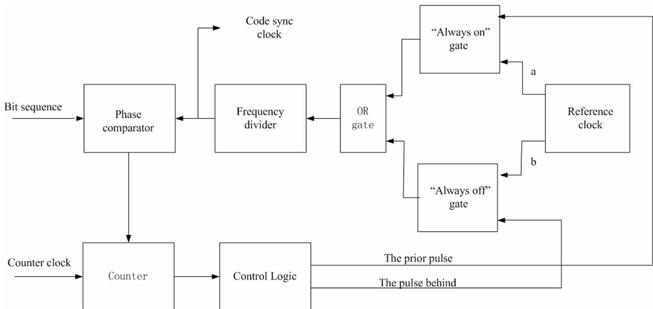
Figure 4 the Improved Structure of Digital PLL
