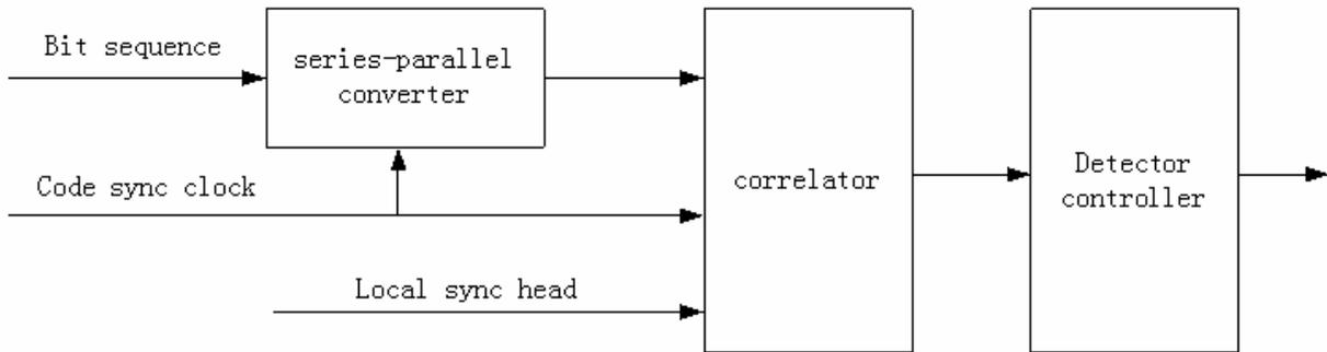
Figure 5 the Frame Synchronization Codeword Detector
