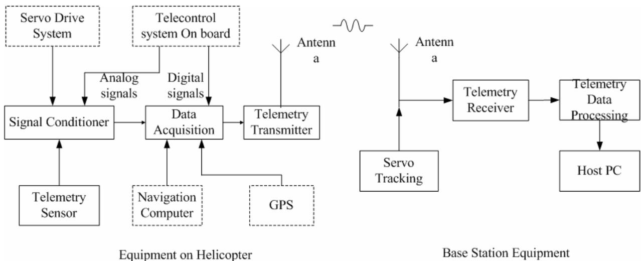
Figure1. Block diagram of telemetry system
