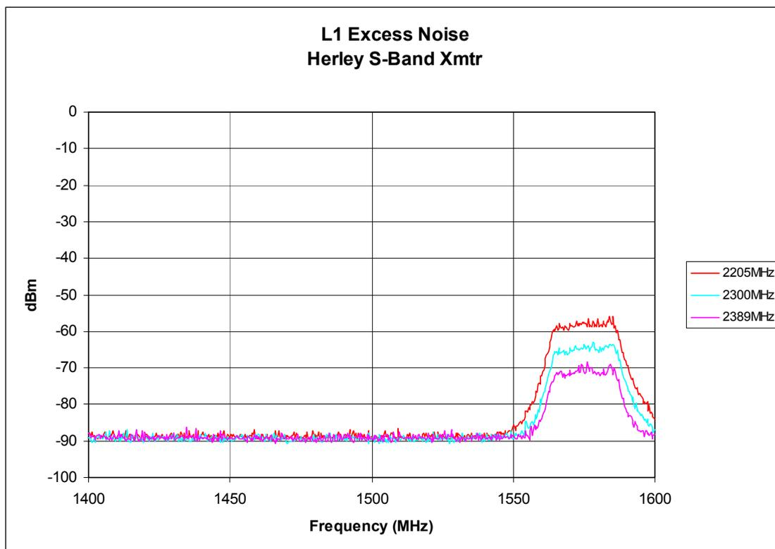
**Figure 3. S-Band FQPSK Transmitter Excess Noise**
