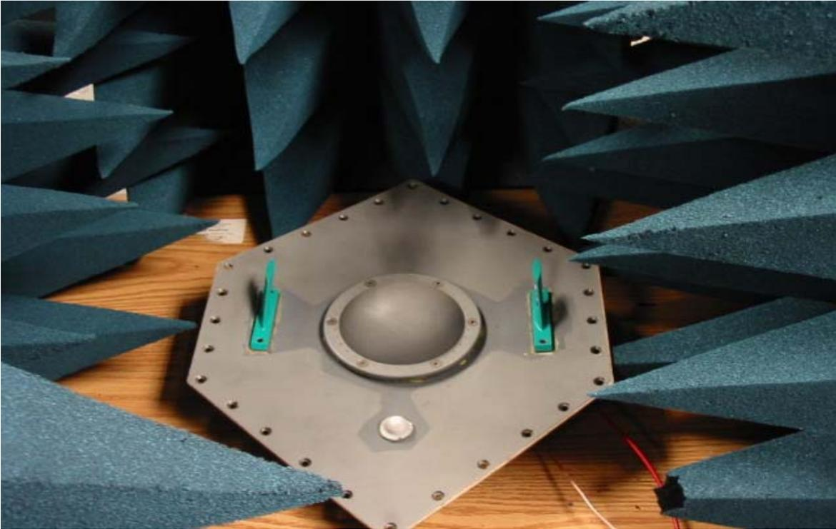
Figure 2. Instrumentation Antenna Plate
