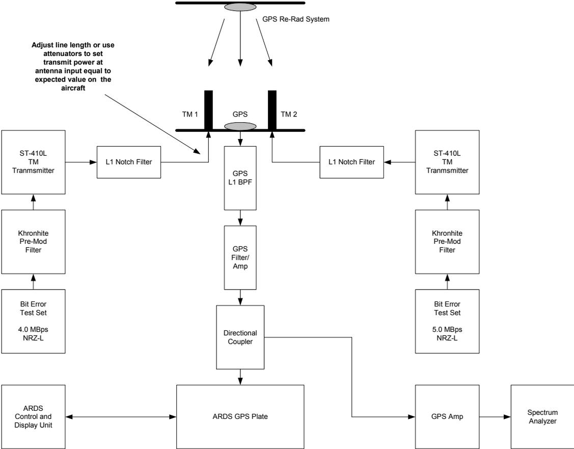
Figure 4. Laboratory Mock and Open-Air Test Configuration
