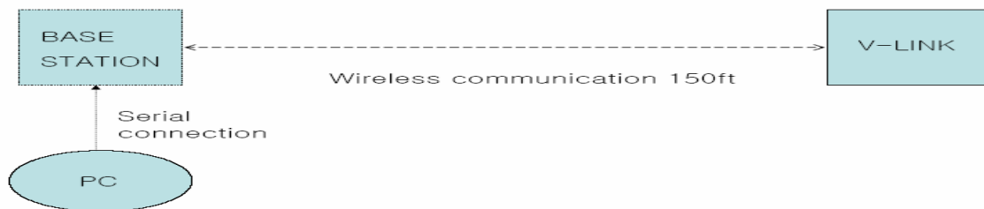
Figure 2. The base station functions as a link between the computer and the V-Link transceivers.
