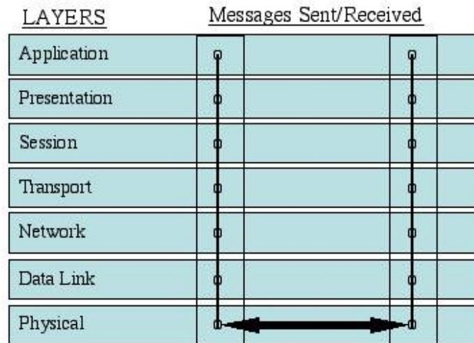
Figure 1. The Open Systems Interconnection 7-Layer Reference Model.
