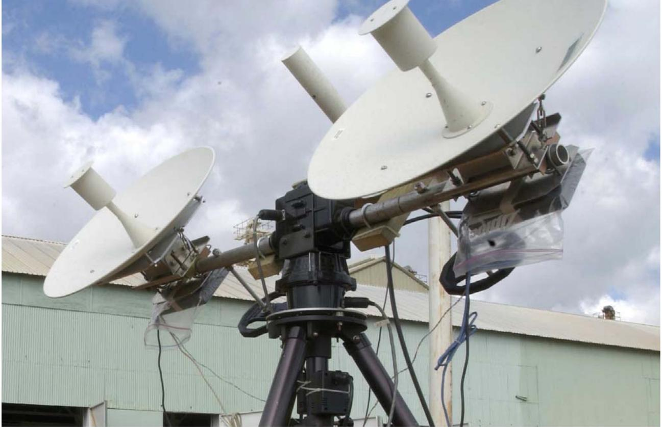
**Figure 3.** Photo shows an array of 3 antennas. The two dishes are WLAN antenna, one for channel 1, and the other channel 11. The S-Band Yagi antenna is used to receive video from the vehicle. This particular rotor shown here has a rotation range of  $450^\circ$  for azimuth and  $180^\circ$  for elevation; and a rotation rate  $6.2^\circ/\text{S}$  for azimuth and  $2.7^\circ/\text{S}$  for elevation.
