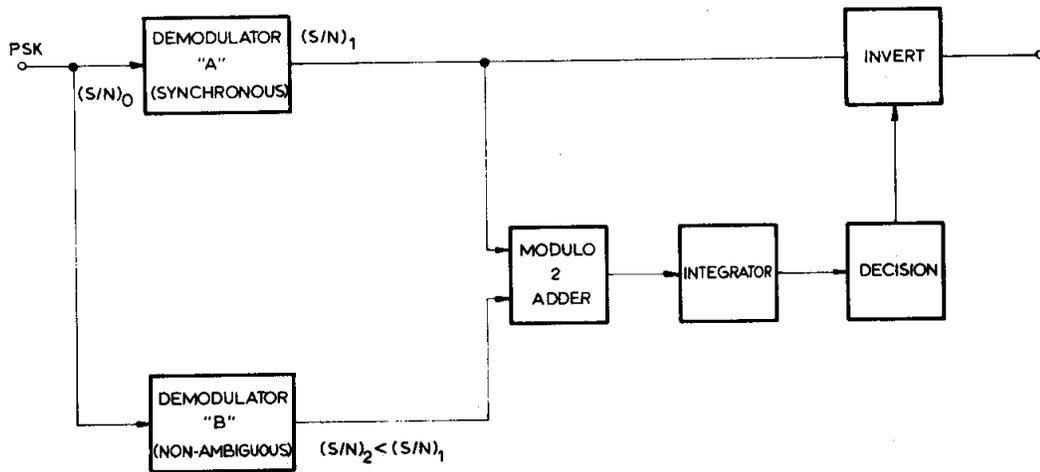
**FIG. 2-2-1 ANTI-AMBIGUITY SYSTEM PRINCIPLE BLOCK DIAGRAM**
