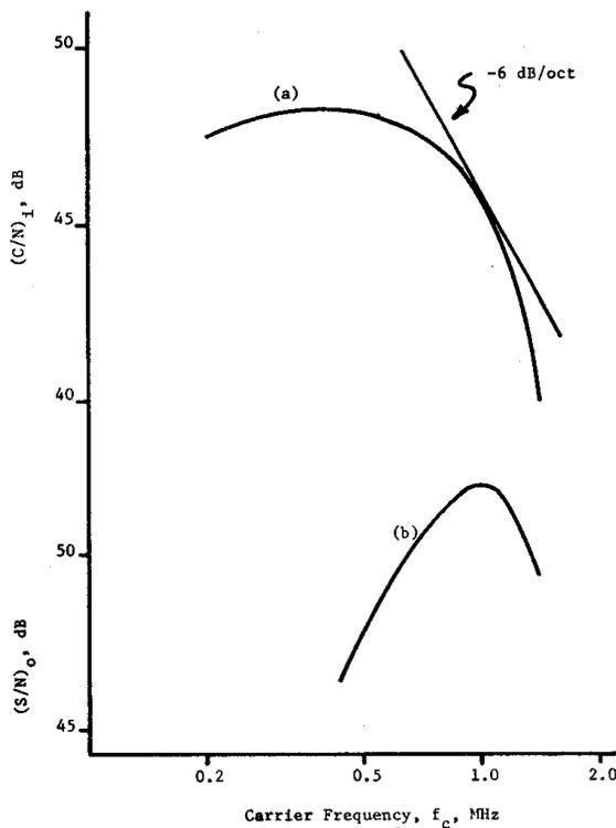
**Fig. 4 - Plot (a) is the Carrier-to-Noise Ratio measured for a tape recorder running at 120 ips with a bandwidth of 256 KHz. Plot (b) is the output Signal-to-Noise Ratio calculated from (a) assuming a frequency deviation of 30%.**
