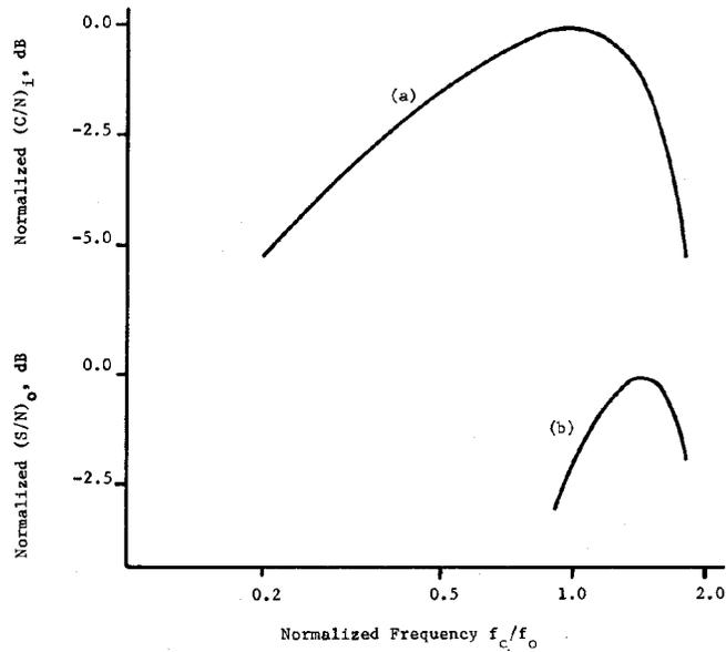
**Fig. 3 - Plots of (a) Input Carrier-to-Noise Ratio and (b) Output Signal-to-Noise Ratio vs. Normalized Carrier Frequency. Input Carrier-to-Noise Ratio is Sinusoidal with Frequency.**
