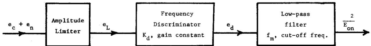
**Fig. 1 - fm System Block Diagram**
