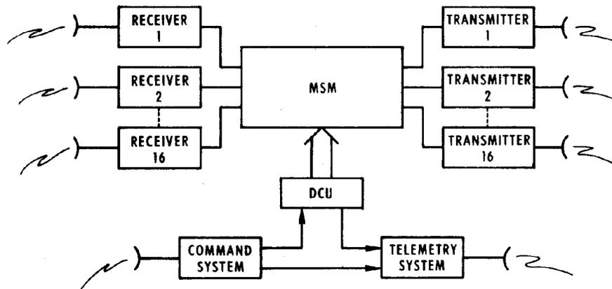
**Fig. 1 - Onboard Distribution System Block Diagram**
