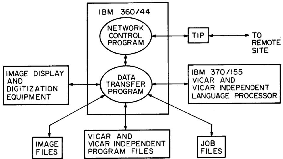
**FIGURE 4. USC/ARPANET IMAGE PROCESSING SYSTEM**
