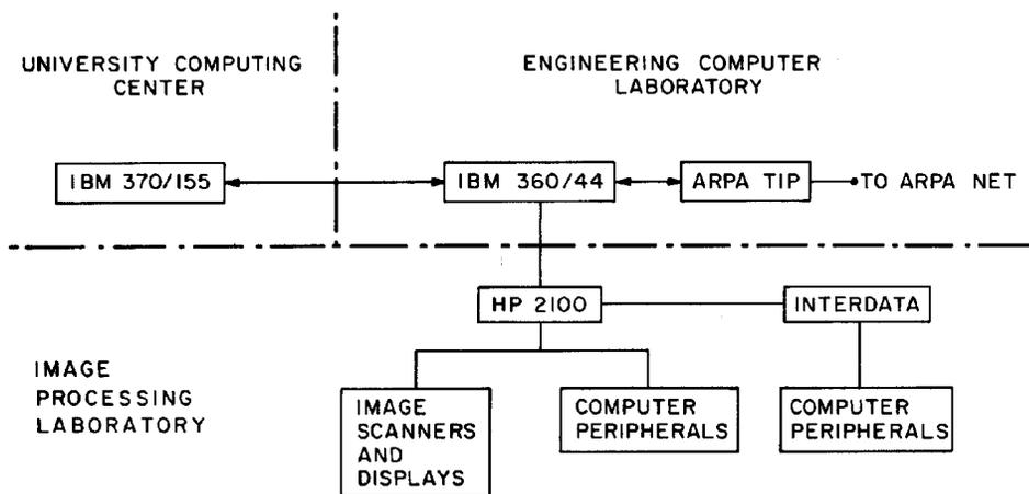
**FIGURE 2. USC IMAGE PROCESSING LABORATORY FACILITIES**
