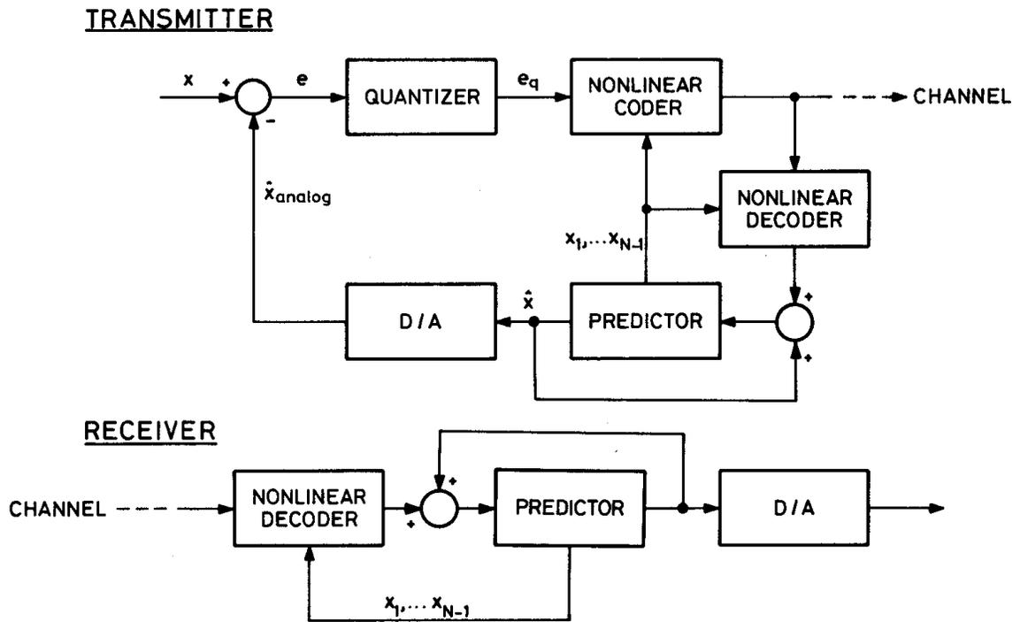
**Fig. 5 - Block diagram of a combined system of linear and non-linear DPCM encoder and decoder**
