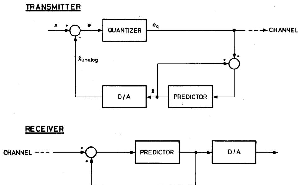
**Fig. 1 - Block diagram of linear DPCM encoder and decoder**
