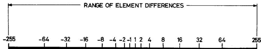
**Fig. 6 - Quantization characteristic of element differences as used for non-linear coder control**
