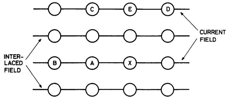
Fig. 3 - Sampling pattern and denotation of elements used for prediction and coder control
