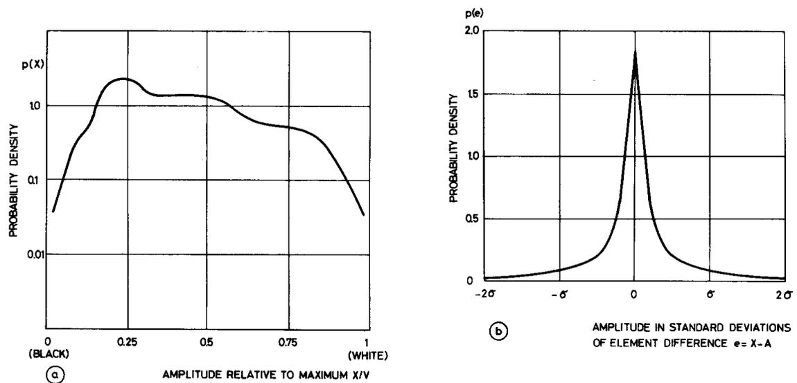
Fig. 4 - Probability distribution of video amplitude and element difference obtained from the four scenes of Fig. 2
