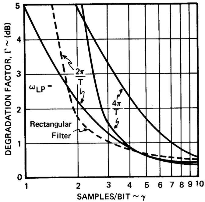
Figure 15 System Degradation Due to Sampling
