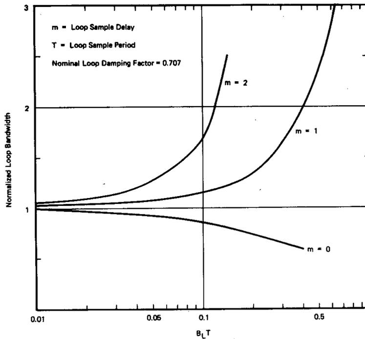
**Figure 13 Increase in Digital Phase-Locked Loop Bandwidth over Design Bandwidth as  $B_L T$  is Increased**
