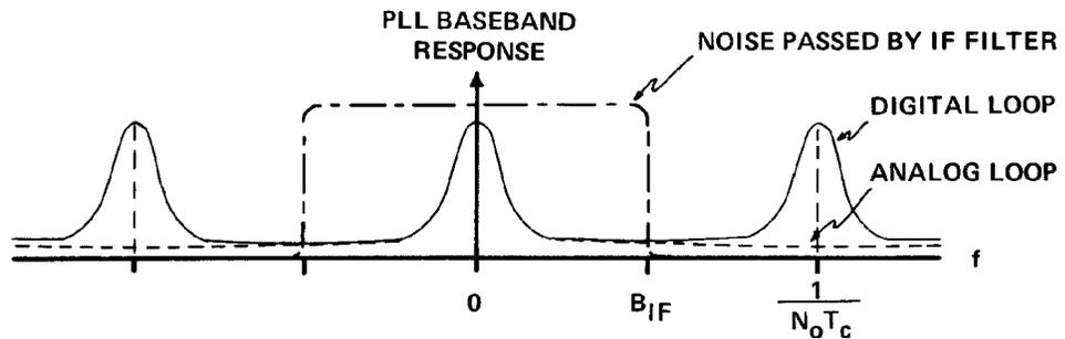
Figure 6 Baseband Response of Analog and Digital PLL's
