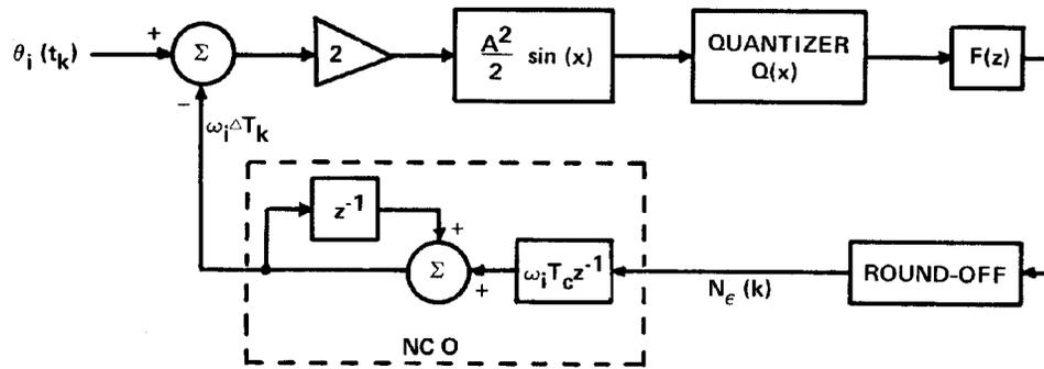
Figure 5 Baseband Model of Digital PLL
