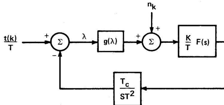
Figure 12 Synchronizer Baseband Model in the "S-Plane"
