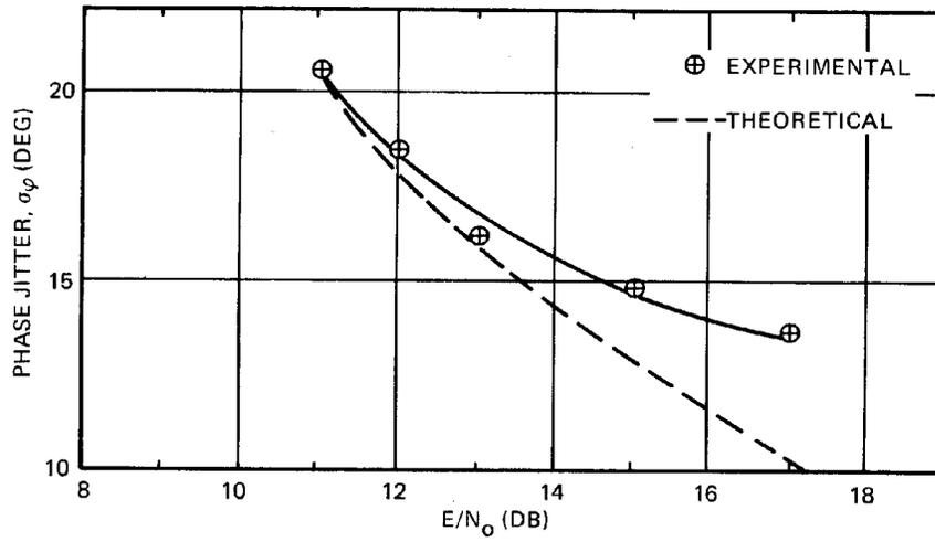
**Figure 18 Carrier Tracking Loop Phase Jitter**
