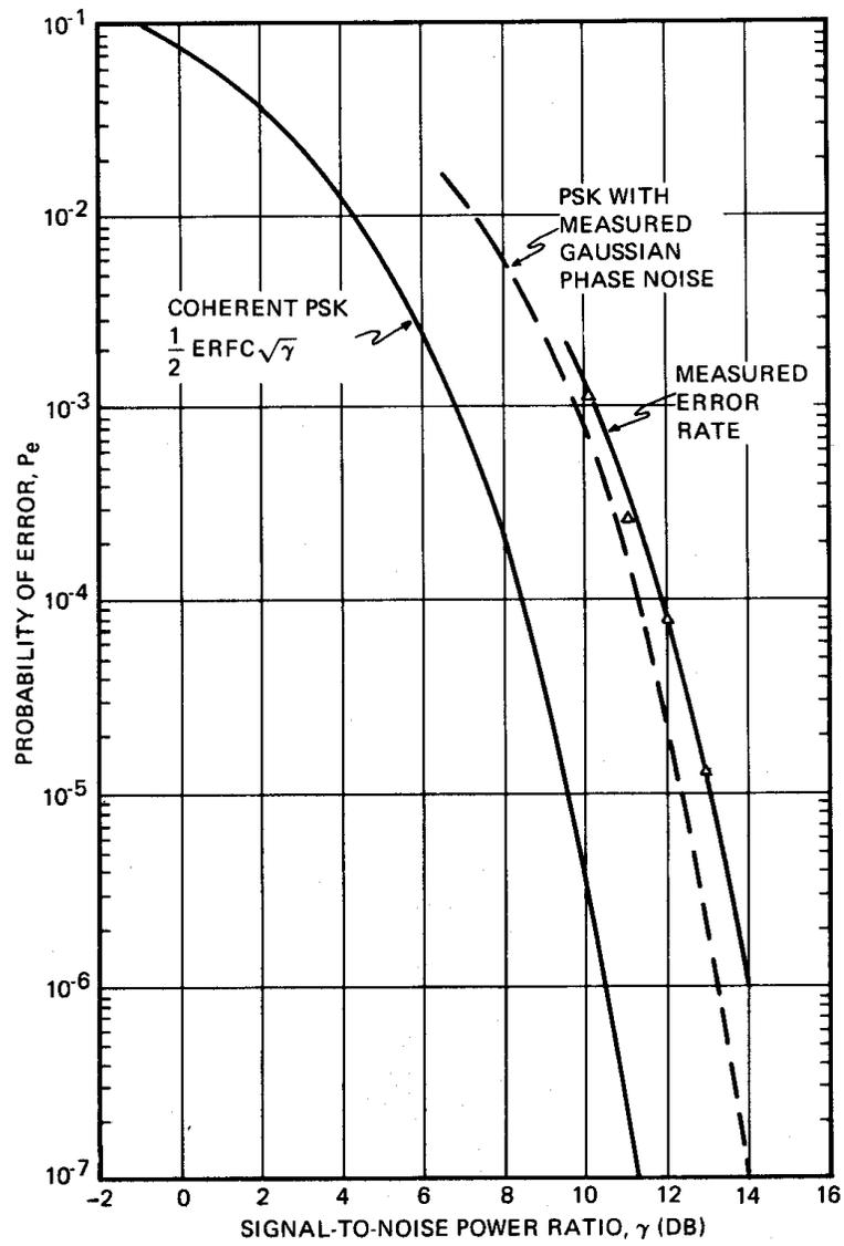
**Figure 20 Bit Error Probability Measurement**
