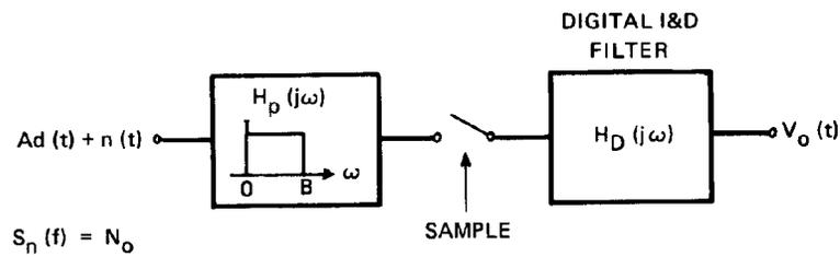
Figure 16 Model of Prefilter and Digital I&D Filter
