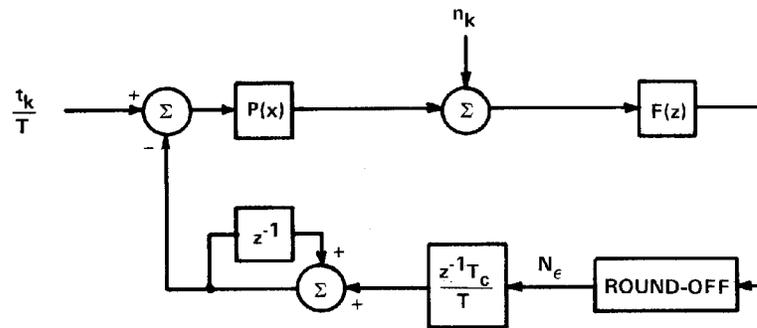
Figure 11 Baseband Model of the Digital Bit Synchronizer
