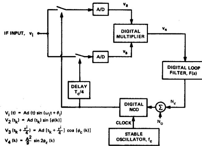
(a) Block diagram of the digital phase-locked loop
