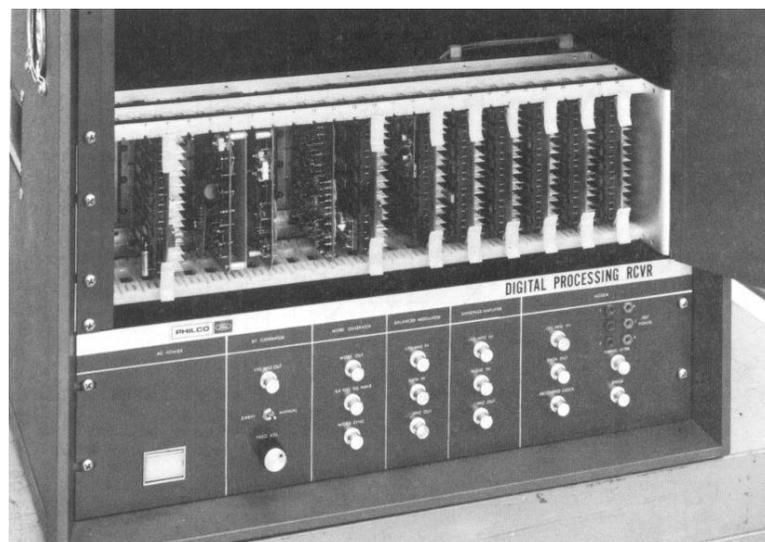
Figure 17 Experimental All-Digital PSK Receiver
