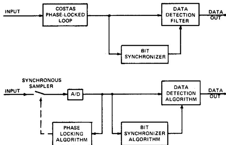
**Figure 1 Conventional Analog PSK Receiver and Equivalent Digital Receiver**
