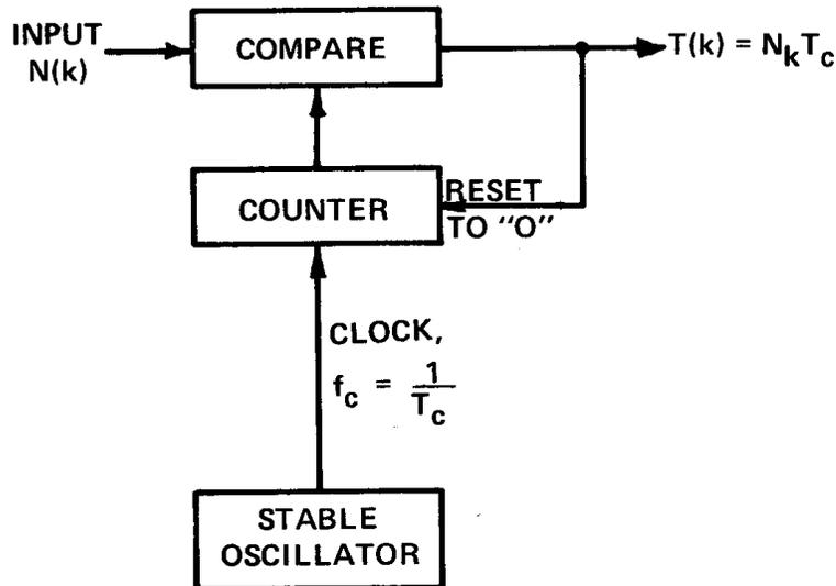
Figure 3 Programmable Divide-by-N Circuit
