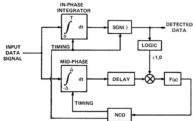
Figure 9 Functional Block Diagram of the Bit Synchronizer
