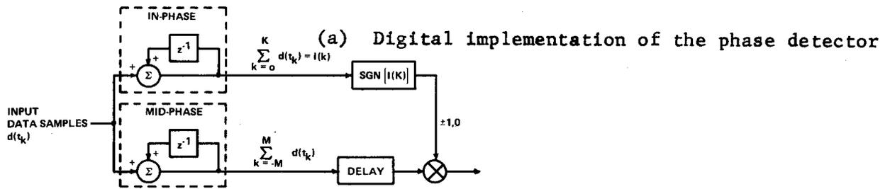
Figure 10 Bit Synchronizer Phase Detector
