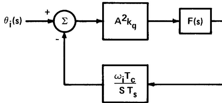
Figure 7 Linearized PLL Baseband Model in the S-Plane
