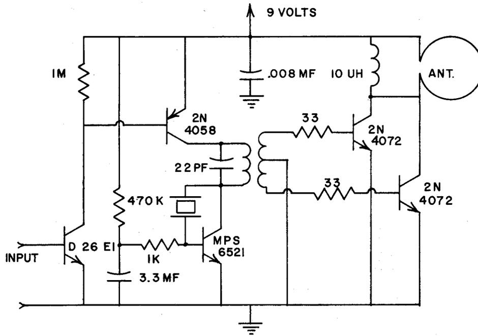
**Fig. 3 - Oscillator-Power Amplifier Circuit Diagram**
