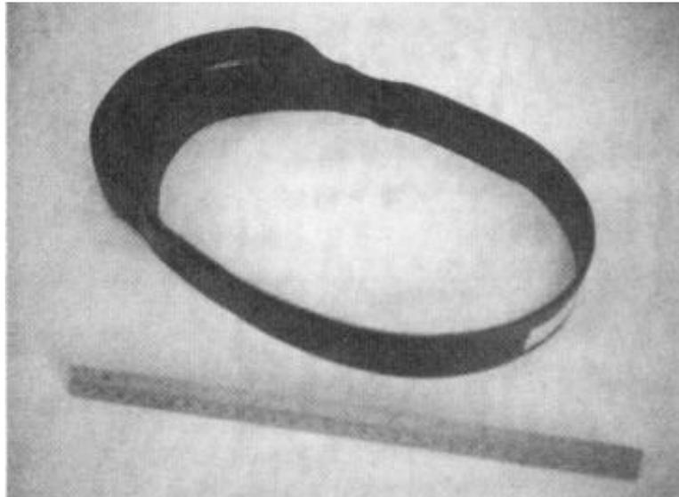
**Fig. 6 - Finished Transmitter With Loop Antenna Built into the Neckband. A One Foot Ruler is Shown in Foreground.**
