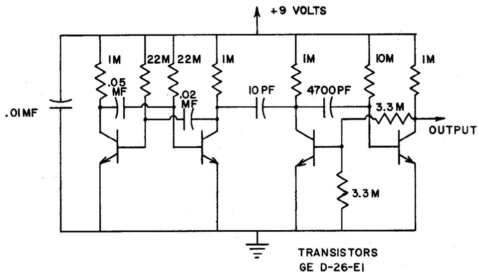
**Fig. 2 - Timing Circuit Diagram**
