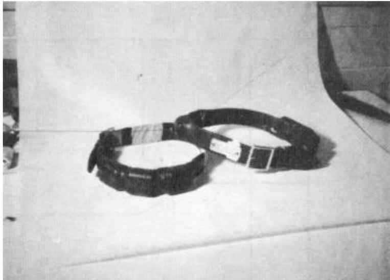
**Fig. 5 - Two Collars with Whip Antennas Ready for Installation on Cow Elk Prior to Transplantation**
