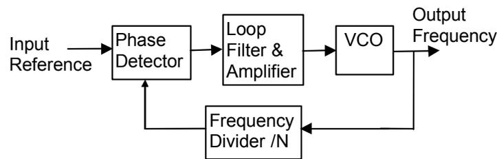
Figure 1. Block diagram of a PLL frequency synthesizer.
