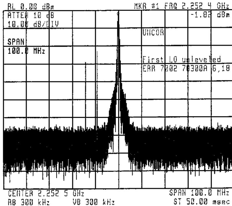
Figure 5. Transmitter output spectrum with digital integrator.
