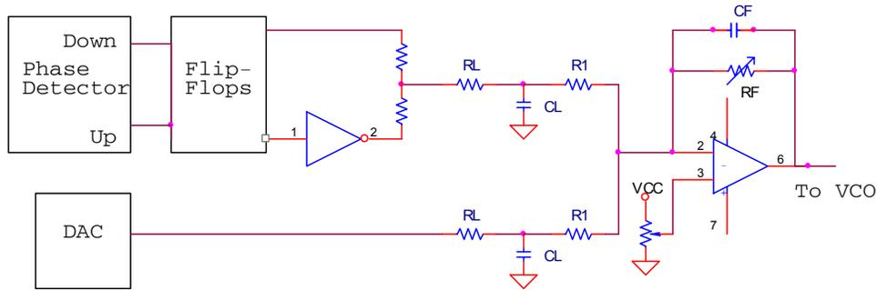
Figure 3. Design of combiner/amplifier/offset block.
