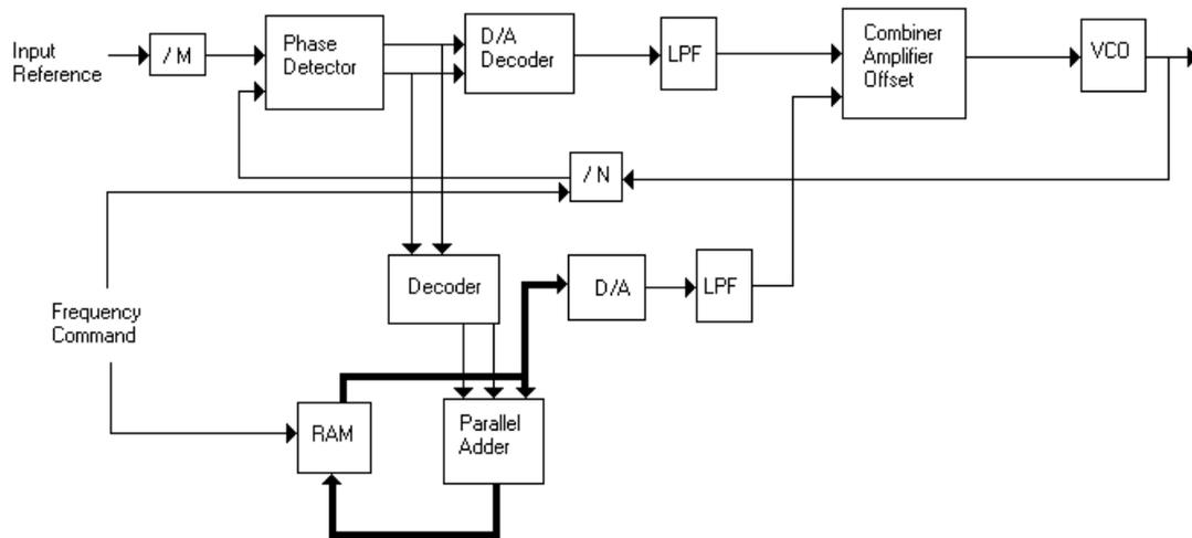
Figure 2. Block diagram of the fast frequency-hopping PLL.
